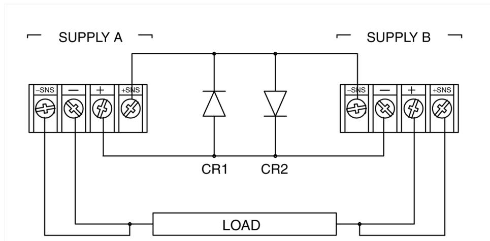
**Figure 4.2** Series Operation With and Without OVP
