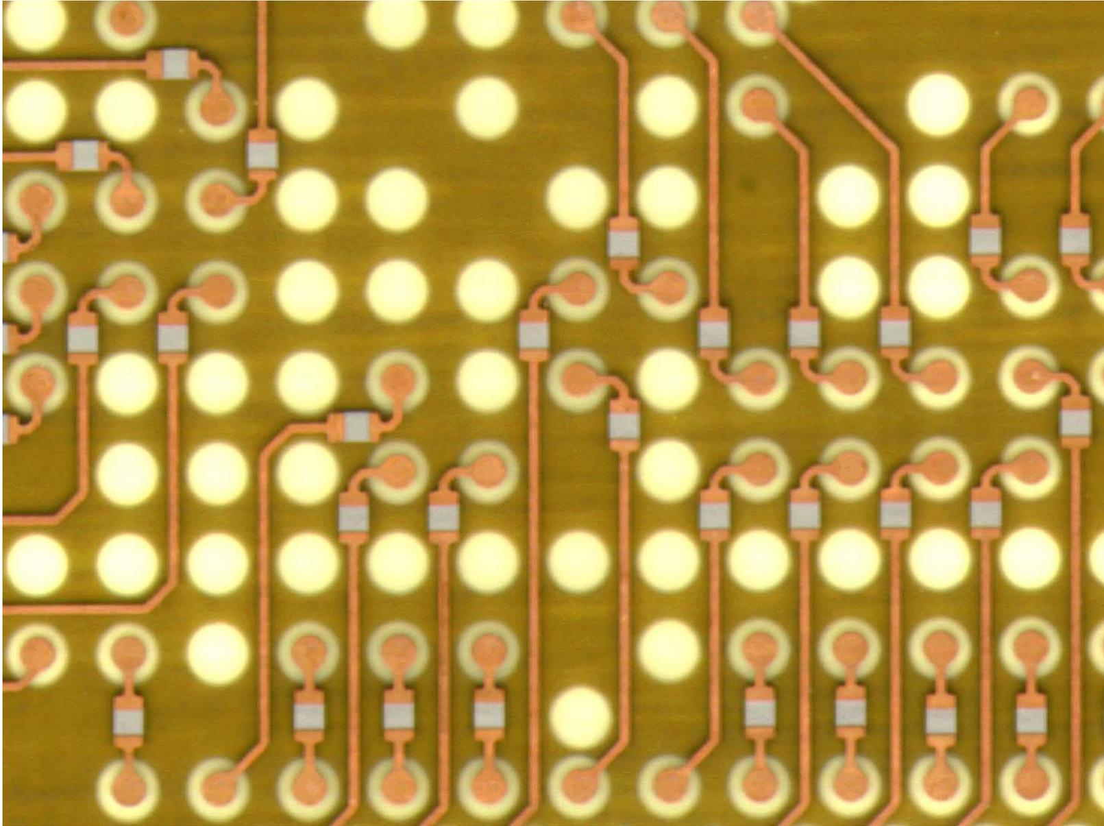
*Series termination resistors for telecom switching card*
