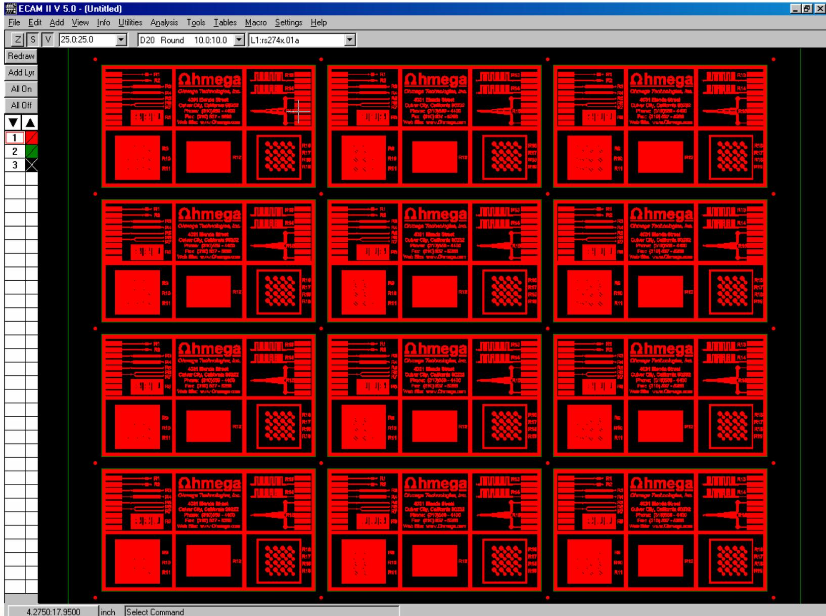
▲ *ECAM Panelized PCB - copper*
