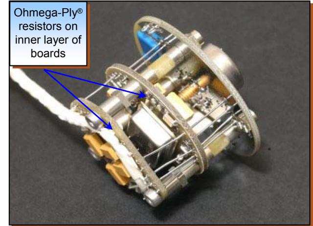
▲ X-Ray Spectrometer (XRS) with Ohmega-Ply<sup>®</sup> resistors
