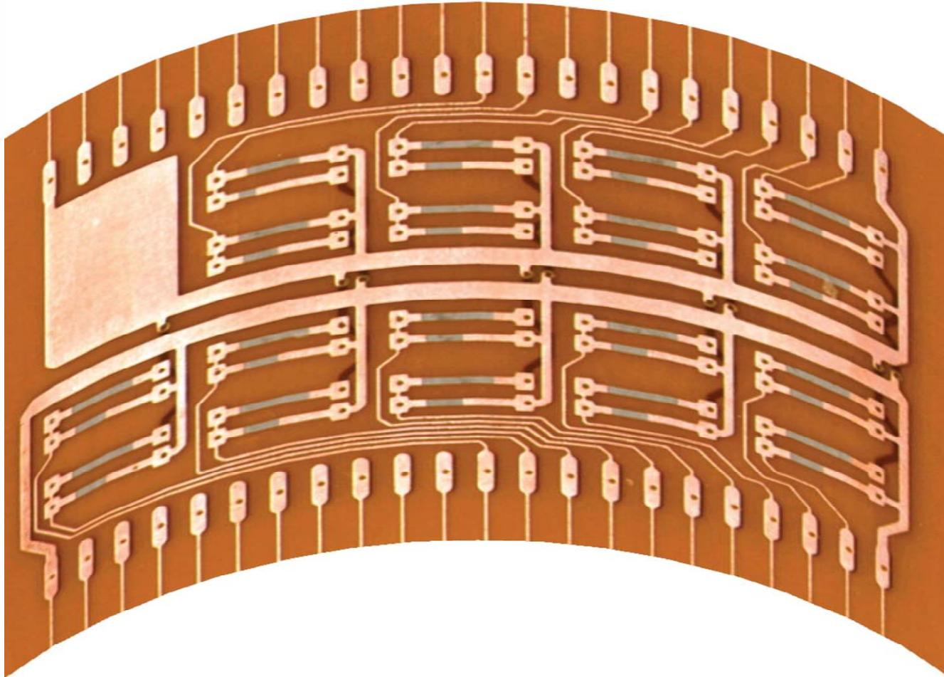
*OhmegaPly<sup>®</sup> Resistors in Flex Circuit*
