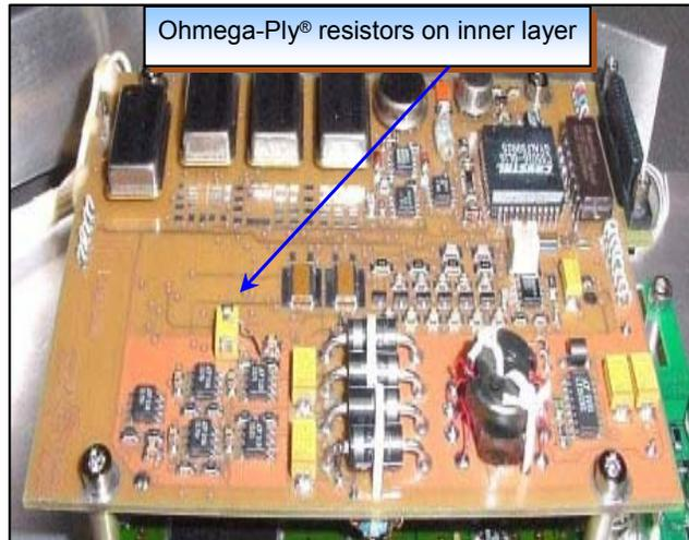
▲ Ohmega-Ply<sup>®</sup> resistors in electronic lander PC board
