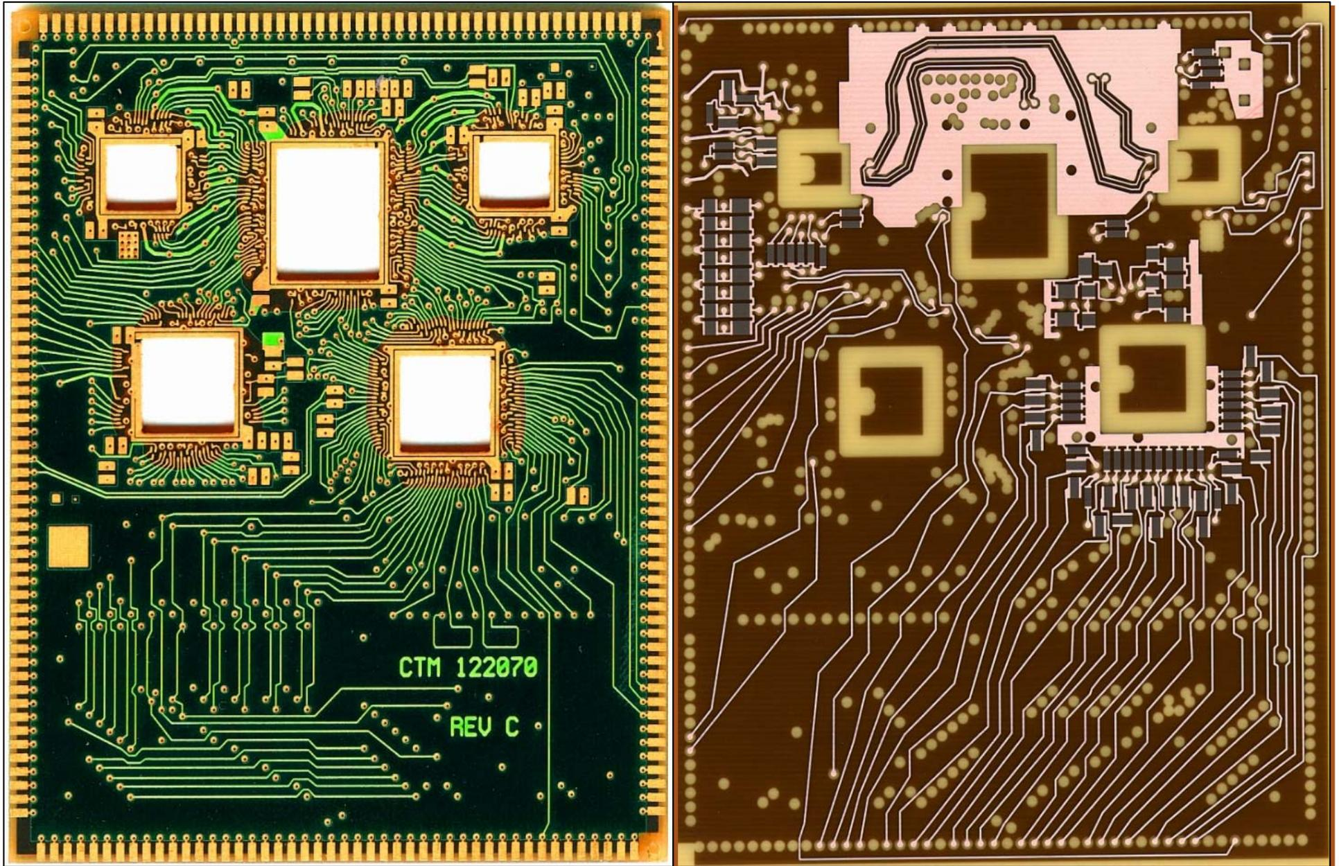
▲ *Buried resistor application – 2" X 3" Probe Card.*
