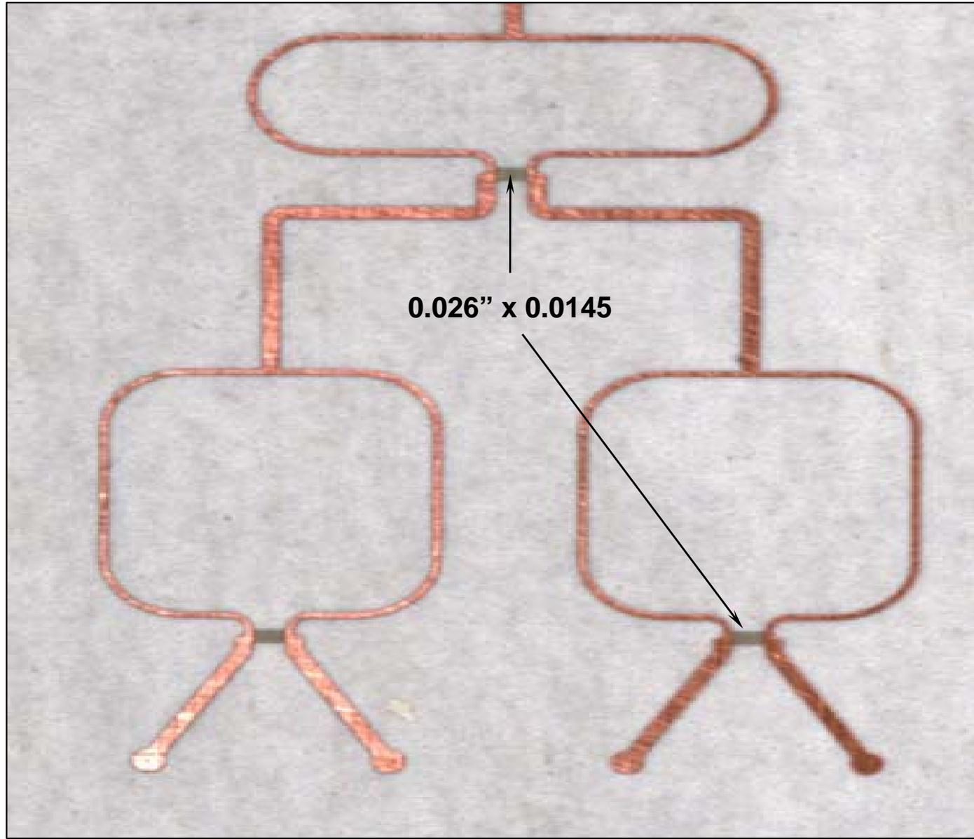
*Enlargement of a four-up array 16-way power divider with 50  $\Omega$ /sq
