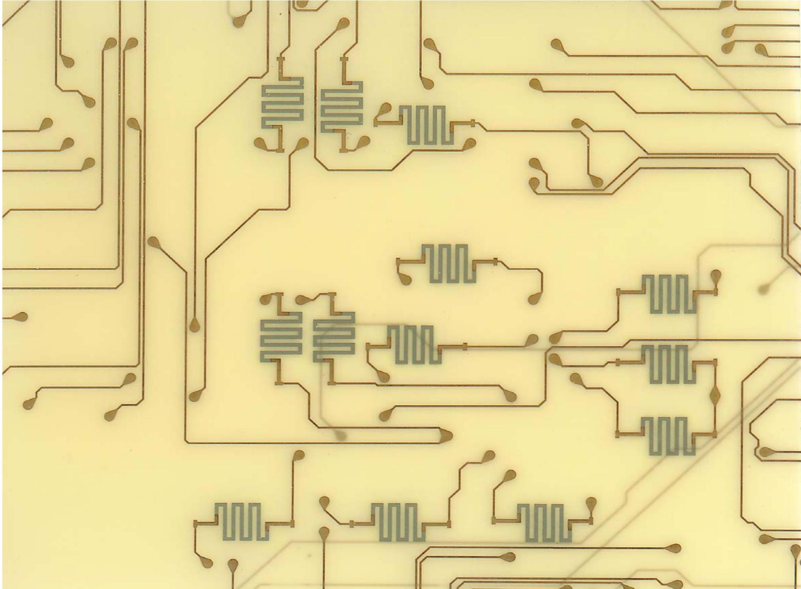
*Pull-up resistors in an avionic application*
