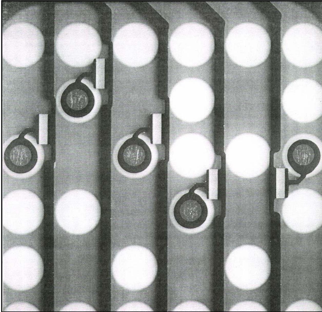
▲ *A server backplane showing thermal/mechanical isolation of OhmegaPly<sup>®</sup> resistors*
