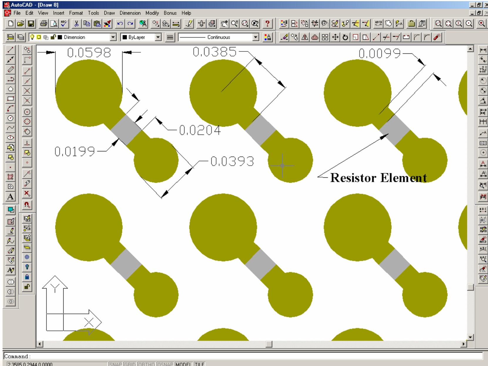
▲ Draw 6 – 50 ohm series termination resistor design.
