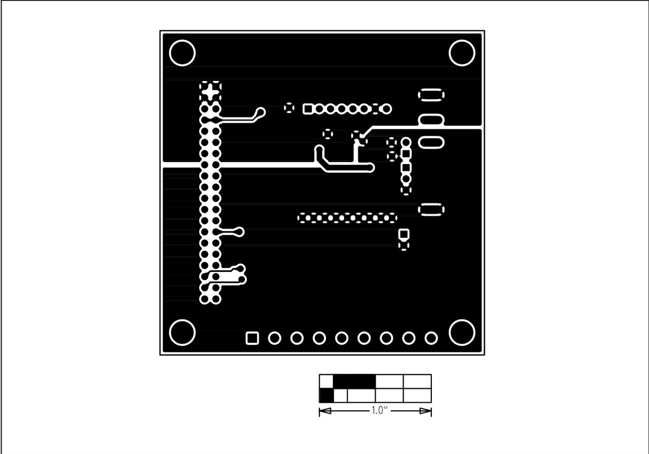
Figure 5. MAX1149 EV Kit PC Board Layout—Solder Side
