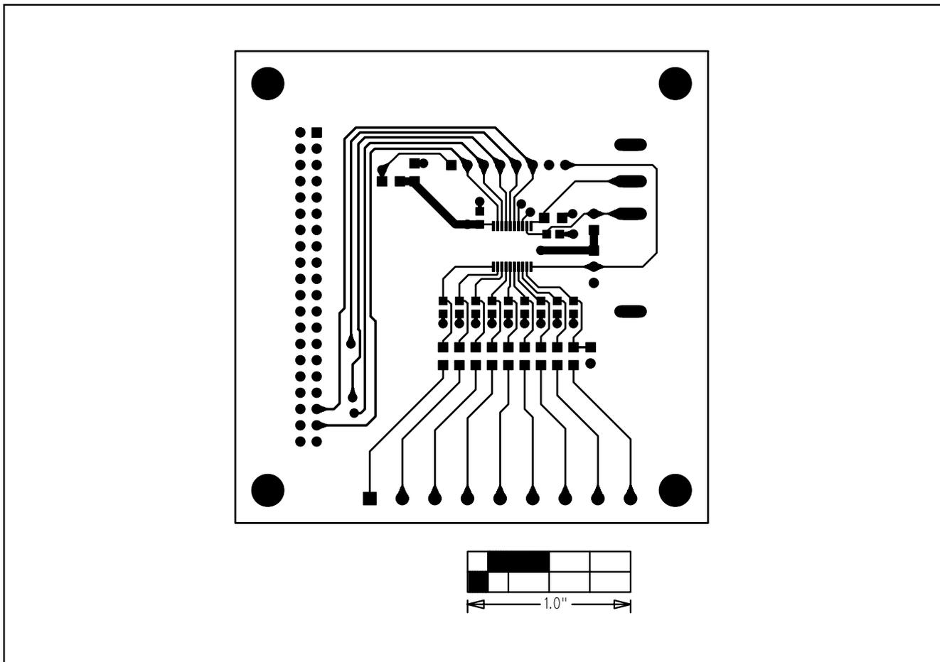
Figure 4. MAX1149 EV Kit PC Board Layout—Component Side
