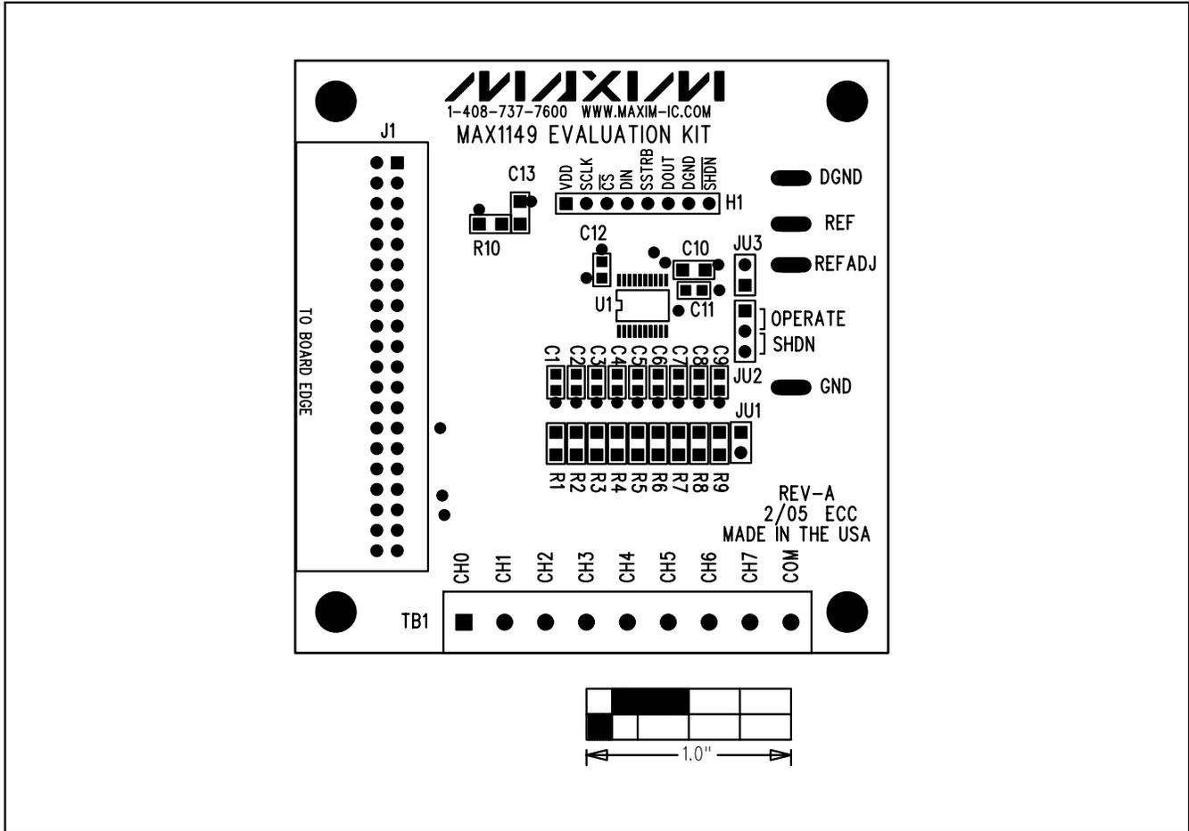
Figure 3. MAX1149 EV Kit Component Placement Guide—Component Side
