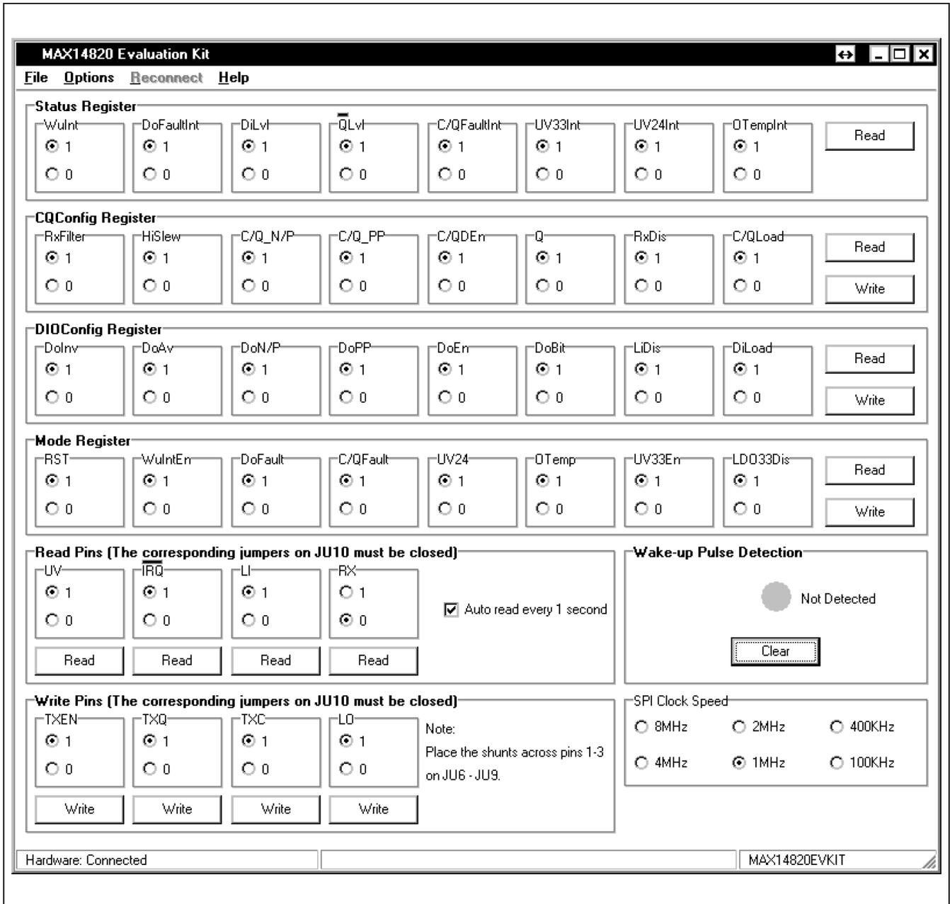
Figure 1. MAX14820 EV Kit Software Main Window
