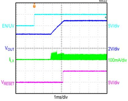
CONDITIONS: 5V OUTPUT, 1kΩ LOAD,  $f_{SW} = 310kHz$
