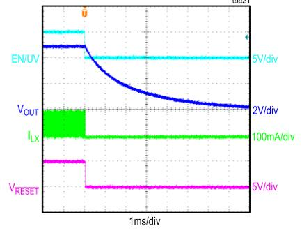
CONDITIONS: 5V OUTPUT, 100Ω LOAD,  $f_{SW} = 310kHz$
