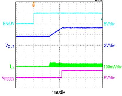
CONDITIONS: 3.3V OUTPUT, 660Ω LOAD,  $f_{SW} = 310kHz$
