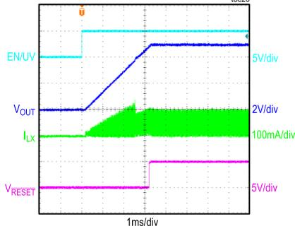
CONDITIONS: 5V OUTPUT, 100Ω LOAD,  $f_{SW} = 310kHz$
