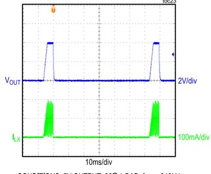
CONDITIONS: 5V OUTPUT, 38Ω LOAD,  $f_{SW} = 310kHz$
