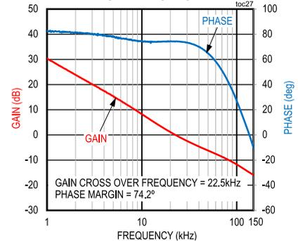
CONDITIONS: 5V OUTPUT, 50mA LOAD,  $f_{SW} = 310kHz$
