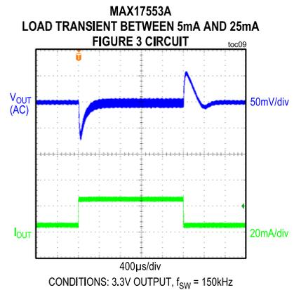
( $V_{IN} = V_{EN/UV} = 24V$ ,  $V_{GND} = 0V$ ,  $T_A = +25^{\circ}C$ , unless otherwise noted. All voltages are referenced to GND, unless otherwise noted.)
