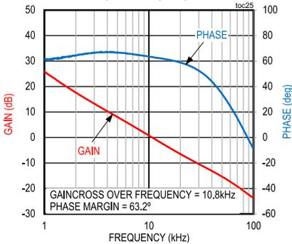
CONDITIONS: 5V OUTPUT, 50mA LOAD,  $f_{SW} = 200kHz$
