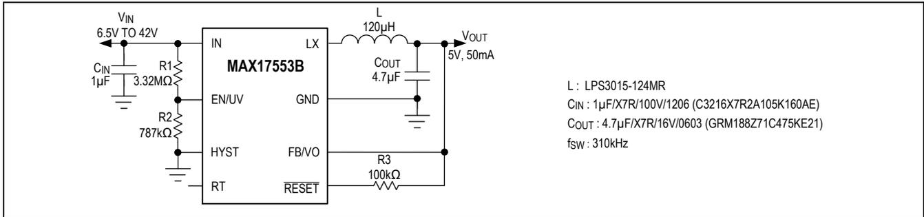
Figure 6. Small-Footprint 5V, 50mA Regulator
