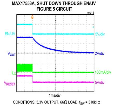
( $V_{IN} = V_{EN/UV} = 24V$ ,  $V_{GND} = 0V$ ,  $T_A = +25^\circ C$ , unless otherwise noted. All voltages are referenced to GND, unless otherwise noted.)
