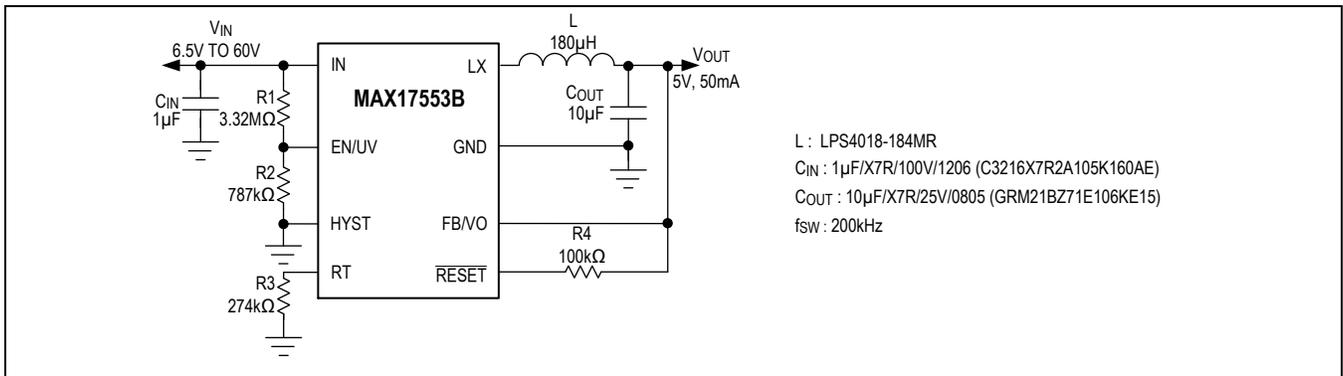
Figure 4. High-Efficiency 5V, 50mA Regulator
