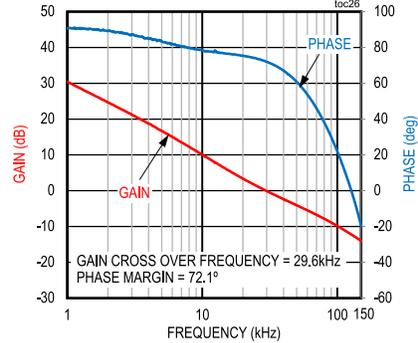
CONDITIONS: 3.3V OUTPUT, 50mA LOAD,  $f_{SW} = 310kHz$
