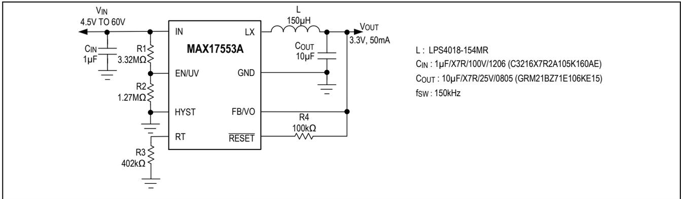
Figure 3. High-Efficiency 3.3V, 50mA Regulator
