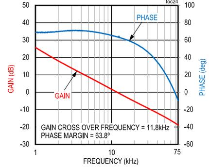
CONDITIONS: 3.3V OUTPUT, 50mA LOAD,  $f_{SW} = 150kHz$
