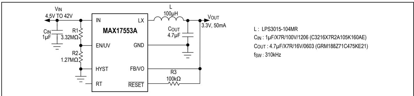
Figure 5. Small-Footprint 3.3V, 50mA Regulator
