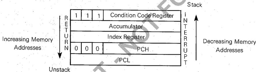
NOTE: Since the stack pointer decrements during pushes, the PCL is stacked first, followed by PCH, etc. Pulling from the stack is in the reverse order.
