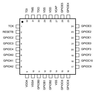
Figure 26. 32-pin LQFP and QFN
