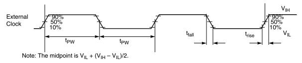
Figure 8. External clock timing
