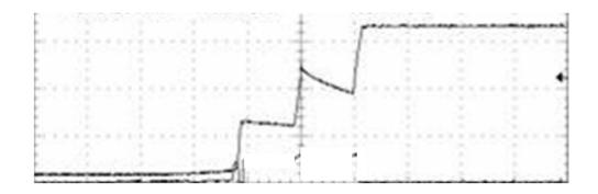
Figure 23. Supply Voltage Drop
