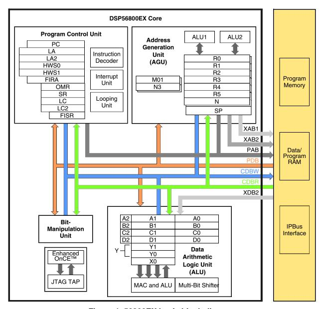
Figure 1. 56800EX basic block diagram
