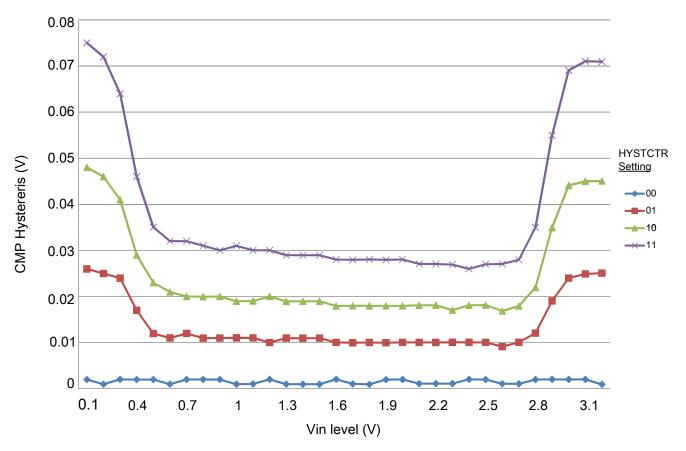
Figure 11. Typical hysteresis vs. Vin level ( $V_{DD} = 3.3 \text{ V}$ , PMODE = 0)
