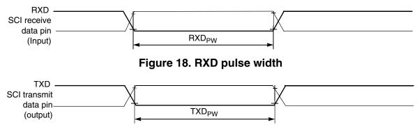
Figure 19. TXD pulse width
