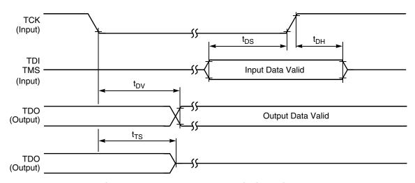
Figure 7. Test access port timing diagram
