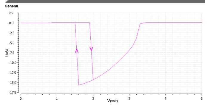
Figure 5. I<sub>IN</sub>/I<sub>OZ</sub> vs. V<sub>IN</sub> (typical; pull-up disabled) (design simulation)
