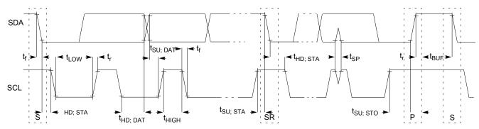
Figure 21. Timing definition for fast and standard mode devices on the I<sup>2</sup>C bus
