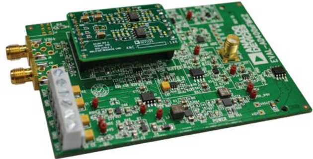
Figure 3. AMC Installed on the EVAL-AD400x-FMCZ
