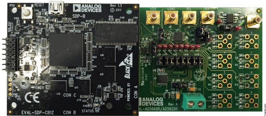
Figure 1. Typical Evaluation Setup of the AD5629R/AD5669R Evaluation Boards
