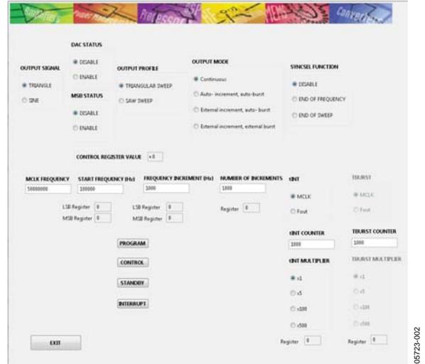
Figure 2. LabVIEW Front End for AD5930
