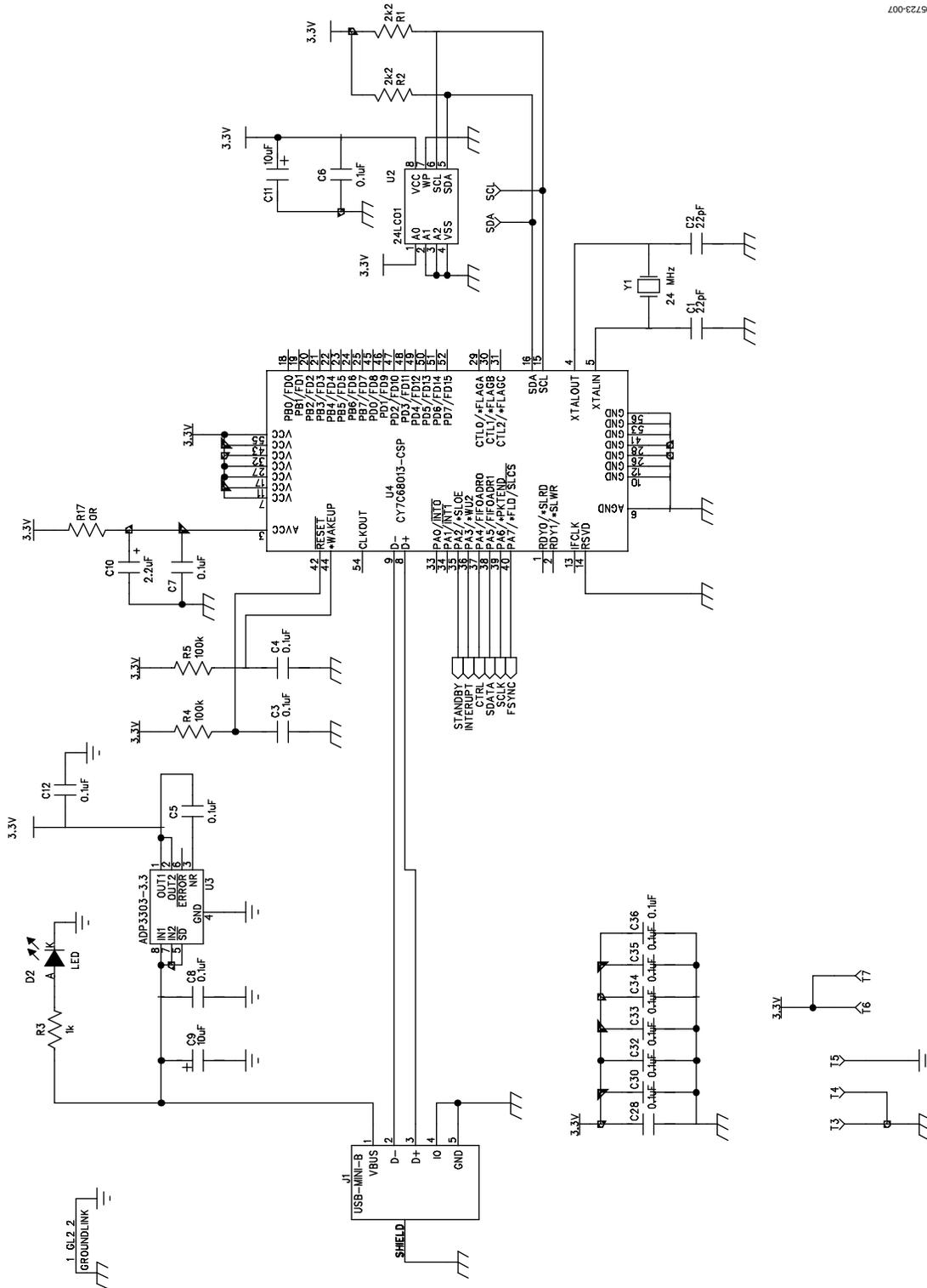
Figure 7. EVAL-AD5930EBZ Schematic, Page 1 of 2
