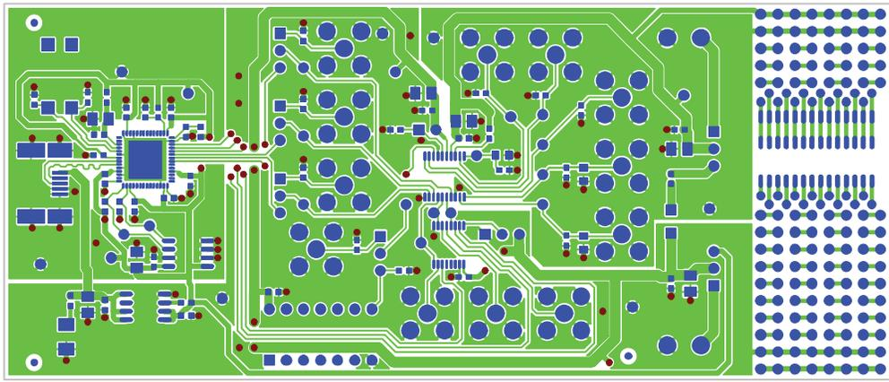
EVAL-AD5930EBZ Rev. A2 – Component Side View Component Side
