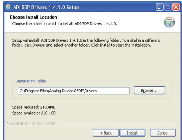
Figure 11. EVAL-SDP-CB1Z Drivers Setup: Selecting the Location for Drivers Installation
