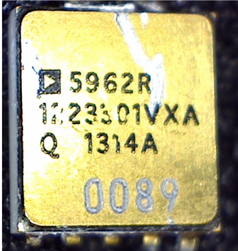
Figure A-1. AD8210 DUT SN 0089 with Package Markings.
