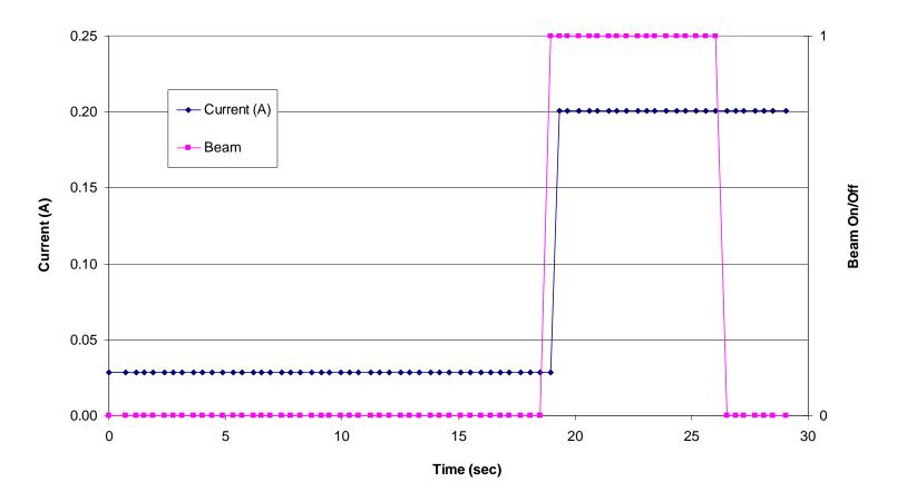
Figure 5.4. Input supply current versus time/fluence for the AD8629 Zero Drift, Single-Supply, Rail-to-Rail, Input/Output Operational Amplifier (run 85, DUT 5, SN2). See Table 4.1 for the details of the test conditions. In this figure the dark blue data points represent the input supply current and the magenta data points represent the beam condition (beam on/beam off). A "0" indicates the shutter is closed (beam off) and a "1" indicates that the shutter is open (beam on).
