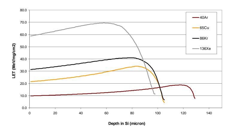
Figure 3.1. Range of the 10 MeV/n Xe, Kr, Cu and Ar beams into silicon. The range to the Bragg Peak for Xe (the shortest range ion used) is approximately  $60 \mu \text{m}$  while the surface LET is approximately 58 MeV-cm2/mg.
