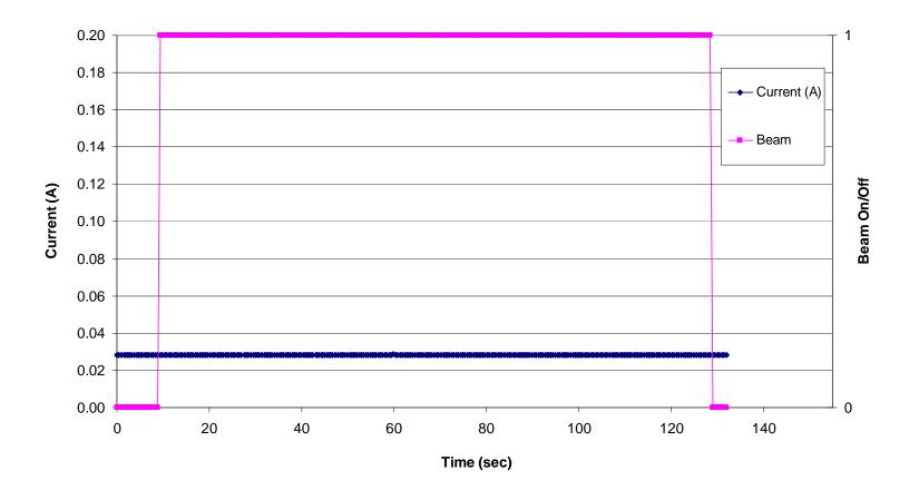
Figure 5.17. Input supply current versus time/fluence for the AD8629 Zero Drift, Single-Supply, Rail-to-Rail, Input/Output Operational Amplifier (run 100, DUT 8, SN12). See Table 4.1 for the details of the test conditions. In this figure the dark blue data points represent the input supply current and the magenta data points represent the beam condition (beam on/beam off). A "0" indicates the shutter is closed (beam off) and a "1" indicates that the shutter is open (beam on).
