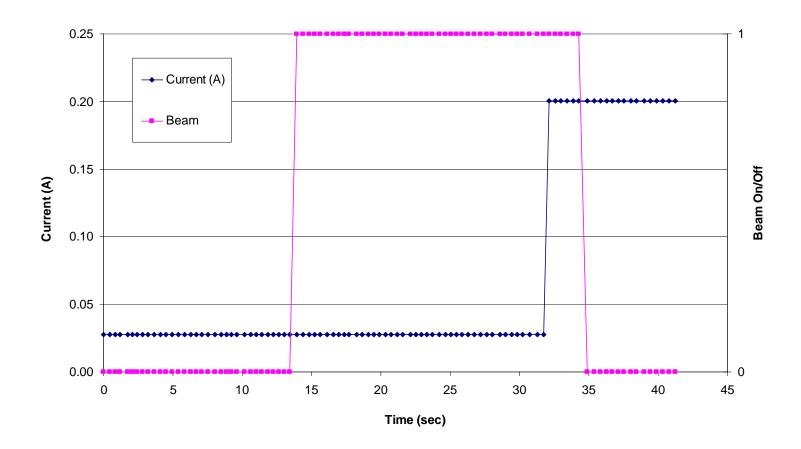
Figure 5.12. Input supply current versus time/fluence for the AD8629 Zero Drift, Single-Supply, Rail-to-Rail, Input/Output Operational Amplifier (run 94, DUT 5, SN2). See Table 4.1 for the details of the test conditions. In this figure the dark blue data points represent the input supply current and the magenta data points represent the beam condition (beam on/beam off). A "0" indicates the shutter is closed (beam off) and a "1" indicates that the shutter is open (beam on).
