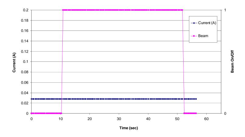
Figure 5.10. Input supply current versus time/fluence for the AD8629 Zero Drift, Single-Supply, Rail-to-Rail, Input/Output Operational Amplifier (run 92, DUT 5, SN2). See Table 4.1 for the details of the test conditions. In this figure the dark blue data points represent the input supply current and the magenta data points represent the beam condition (beam on/beam off). A "0" indicates the shutter is closed (beam off) and a "1" indicates that the shutter is open (beam on).
