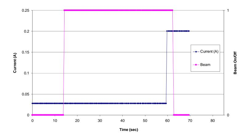
Figure 5.14. Input supply current versus time/fluence for the AD8629 Zero Drift, Single-Supply, Rail-to-Rail, Input/Output Operational Amplifier (run 96, DUT 5, SN2). See Table 4.1 for the details of the test conditions. In this figure the dark blue data points represent the input supply current and the magenta data points represent the beam condition (beam on/beam off). A "0" indicates the shutter is closed (beam off) and a "1" indicates that the shutter is open (beam on).
