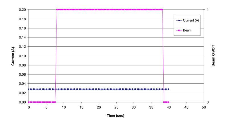
Figure 5.2. Input supply current versus time/fluence for the AD8629 Zero Drift, Single-Supply, Rail-to-Rail, Input/Output Operational Amplifier (run 83, DUT 6, SN3). See Table 4.1 for the details of the test conditions. In this figure the dark blue data points represent the input supply current and the magenta data points represent the beam condition (beam on/beam off). A "0" indicates the shutter is closed (beam off) and a "1" indicates that the shutter is open (beam on).
