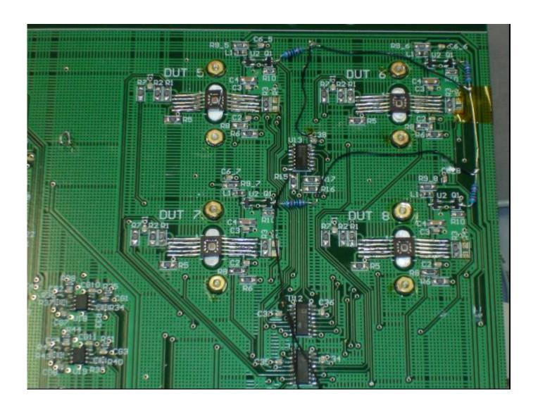
Figure 3.1. Single event test board that was mounted on the test stage at Berkeley. The board has four units-under-test (labeled as DUTs 5, 6, 7 and 8) mounted simultaneously to minimize vacuum breaks during testing. There is also a heater plate mounted to the backside of the board to provide the elevated temperature required for this testing.
