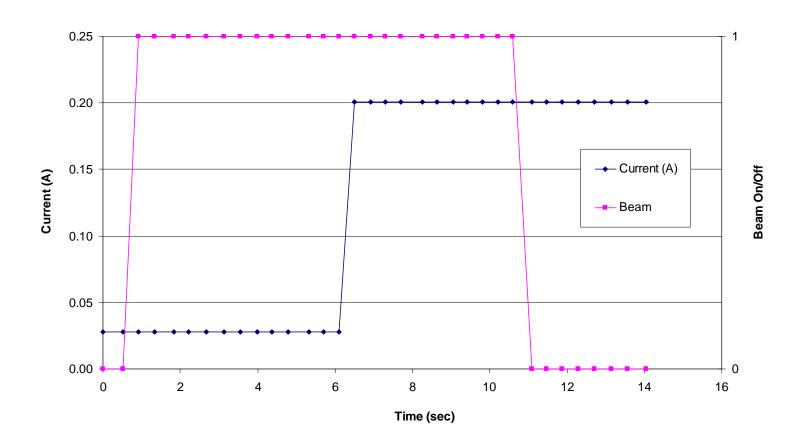
Figure 5.23. Input supply current versus time/fluence for the AD8629 Zero Drift, Single-Supply, Rail-to-Rail, Input/Output Operational Amplifier (run 106, DUT 7, SN11). See Table 4.1 for the details of the test conditions. In this figure the dark blue data points represent the input supply current and the magenta data points represent the beam condition (beam on/beam off). A "0" indicates the shutter is closed (beam off) and a "1" indicates that the shutter is open (beam on).
