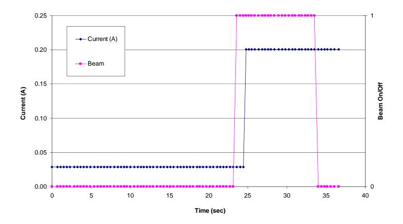
Figure 5.18. Input supply current versus time/fluence for the AD8629 Zero Drift, Single-Supply, Rail-to-Rail, Input/Output Operational Amplifier (run 101, DUT 8, SN12). See Table 4.1 for the details of the test conditions. In this figure the dark blue data points represent the input supply current and the magenta data points represent the beam condition (beam on/beam off). A "0" indicates the shutter is closed (beam off) and a "1" indicates that the shutter is open (beam on).
