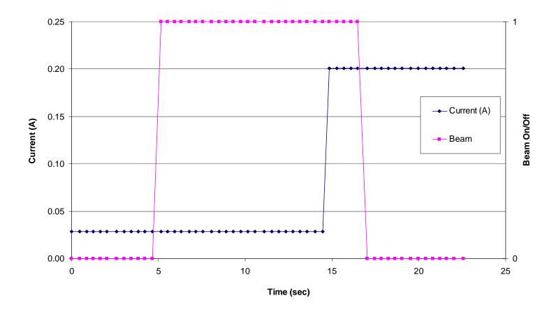
Figure 5.21. Input supply current versus time/fluence for the AD8629 Zero Drift, Single-Supply, Rail-to-Rail, Input/Output Operational Amplifier (run 104, DUT 8, SN12). See Table 4.1 for the details of the test conditions. In this figure the dark blue data points represent the input supply current and the magenta data points represent the beam condition (beam on/beam off). A "0" indicates the shutter is closed (beam off) and a "1" indicates that the shutter is open (beam on).
