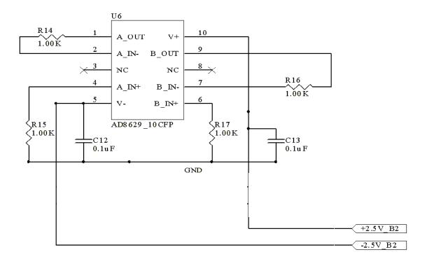
Figure B.1. Schematic drawing of the bias configuration used for the SEL test described in this final report.
