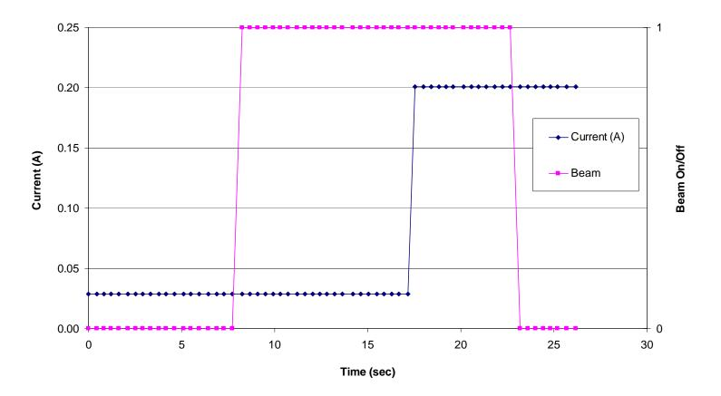
Figure 5.22. Input supply current versus time/fluence for the AD8629 Zero Drift, Single-Supply, Rail-to-Rail, Input/Output Operational Amplifier (run 105, DUT 8, SN12). See Table 4.1 for the details of the test conditions. In this figure the dark blue data points represent the input supply current and the magenta data points represent the beam condition (beam on/beam off). A "0" indicates the shutter is closed (beam off) and a "1" indicates that the shutter is open (beam on).
