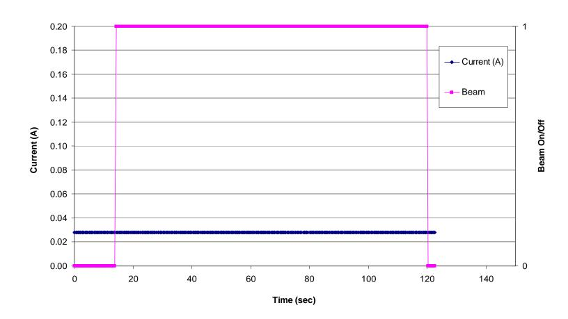
Figure 5.15. Input supply current versus time/fluence for the AD8629 Zero Drift, Single-Supply, Rail-to-Rail, Input/Output Operational Amplifier (run 97, DUT 6, SN3). See Table 4.1 for the details of the test conditions. In this figure the dark blue data points represent the input supply current and the magenta data points represent the beam condition (beam on/beam off). A "0" indicates the shutter is closed (beam off) and a "1" indicates that the shutter is open (beam on).
