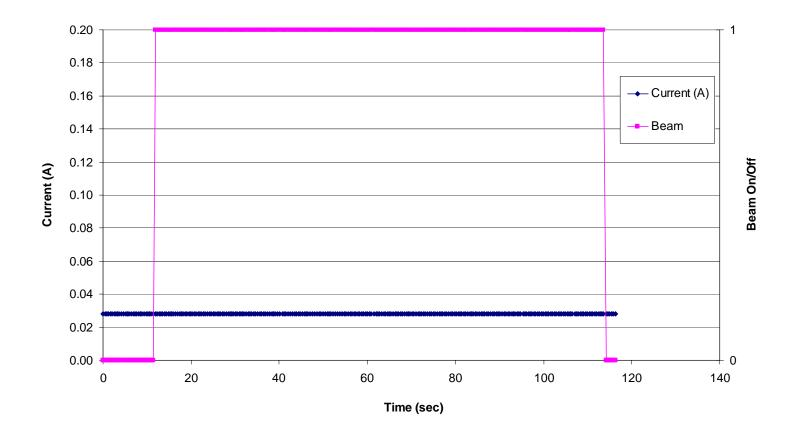
Figure 5.16. Input supply current versus time/fluence for the AD8629 Zero Drift, Single-Supply, Rail-to-Rail, Input/Output Operational Amplifier (run 98, DUT 6, SN3). See Table 4.1 for the details of the test conditions. In this figure the dark blue data points represent the input supply current and the magenta data points represent the beam condition (beam on/beam off). A "0" indicates the shutter is closed (beam off) and a "1" indicates that the shutter is open (beam on).
