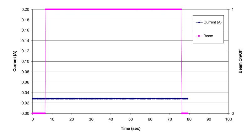
Figure 5.3. Input supply current versus time/fluence for the AD8629 Zero Drift, Single-Supply, Rail-to-Rail, Input/Output Operational Amplifier (run 84, DUT 5, SN2). See Table 4.1 for the details of the test conditions. In this figure the dark blue data points represent the input supply current and the magenta data points represent the beam condition (beam on/beam off). A "0" indicates the shutter is closed (beam off) and a "1" indicates that the shutter is open (beam on).
