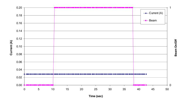
Figure 5.5. Input supply current versus time/fluence for the AD8629 Zero Drift, Single-Supply, Rail-to-Rail, Input/Output Operational Amplifier (run 86, DUT 5, SN2). See Table 4.1 for the details of the test conditions. In this figure the dark blue data points represent the input supply current and the magenta data points represent the beam condition (beam on/beam off). A "0" indicates the shutter is closed (beam off) and a "1" indicates that the shutter is open (beam on).
