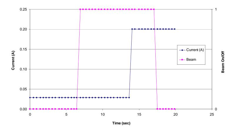
Figure 5.19. Input supply current versus time/fluence for the AD8629 Zero Drift, Single-Supply, Rail-to-Rail, Input/Output Operational Amplifier (run 102, DUT 8, SN12). See Table 4.1 for the details of the test conditions. In this figure the dark blue data points represent the input supply current and the magenta data points represent the beam condition (beam on/beam off). A "0" indicates the shutter is closed (beam off) and a "1" indicates that the shutter is open (beam on).
