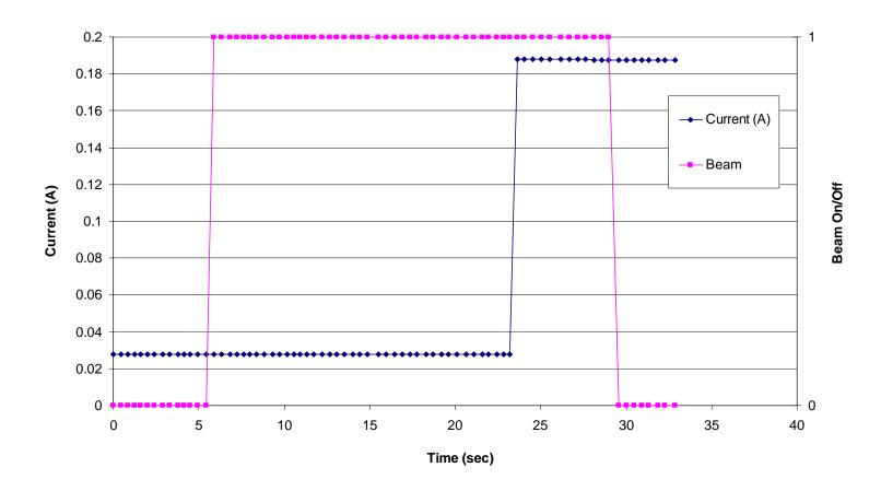
Figure 5.24. Input supply current versus time/fluence for the AD8629 Zero Drift, Single-Supply, Rail-to-Rail, Input/Output Operational Amplifier (run 107, DUT 7, SN11). See Table 4.1 for the details of the test conditions. In this figure the dark blue data points represent the input supply current and the magenta data points represent the beam condition (beam on/beam off). A "0" indicates the shutter is closed (beam off) and a "1" indicates that the shutter is open (beam on).
