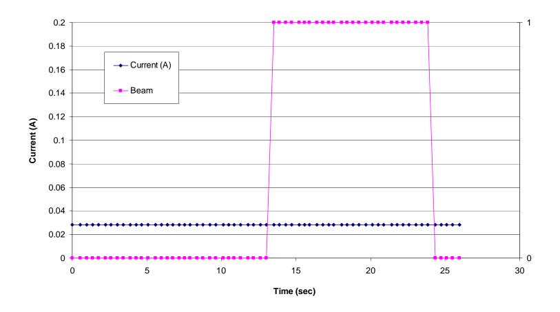
Figure 5.7. Input supply current versus time/fluence for the AD8629 Zero Drift, Single-Supply, Rail-to-Rail, Input/Output Operational Amplifier (run 89, DUT 7, SN11). See Table 4.1 for the details of the test conditions. In this figure the dark blue data points represent the input supply current and the magenta data points represent the beam condition (beam on/beam off). A "0" indicates the shutter is closed (beam off) and a "1" indicates that the shutter is open (beam on).
