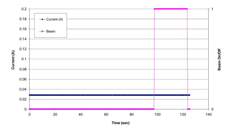
Figure 5.6. Input supply current versus time/fluence for the AD8629 Zero Drift, Single-Supply, Rail-to-Rail, Input/Output Operational Amplifier (run 88, DUT 5, SN2). See Table 4.1 for the details of the test conditions. In this figure the dark blue data points represent the input supply current and the magenta data points represent the beam condition (beam on/beam off). A "0" indicates the shutter is closed (beam off) and a "1" indicates that the shutter is open (beam on).
