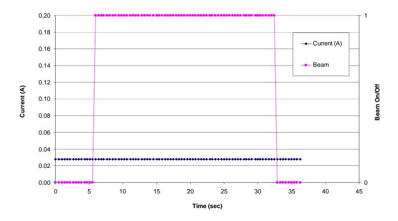
Figure 5.8. Input supply current versus time/fluence for the AD8629 Zero Drift, Single-Supply, Rail-to-Rail, Input/Output Operational Amplifier (run 90, DUT 7, SN11). See Table 4.1 for the details of the test conditions. In this figure the dark blue data points represent the input supply current and the magenta data points represent the beam condition (beam on/beam off). A "0" indicates the shutter is closed (beam off) and a "1" indicates that the shutter is open (beam on).
