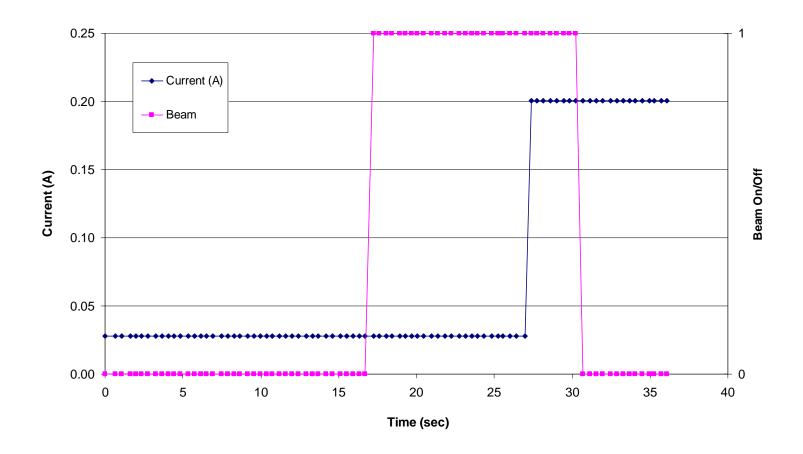
Figure 5.11. Input supply current versus time/fluence for the AD8629 Zero Drift, Single-Supply, Rail-to-Rail, Input/Output Operational Amplifier (run 93, DUT 5, SN2). See Table 4.1 for the details of the test conditions. In this figure the dark blue data points represent the input supply current and the magenta data points represent the beam condition (beam on/beam off). A "0" indicates the shutter is closed (beam off) and a "1" indicates that the shutter is open (beam on).
