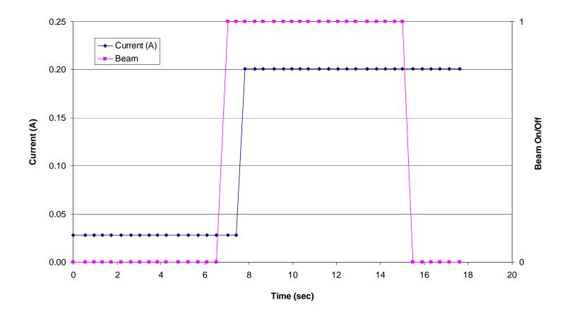
Figure 5.13. Input supply current versus time/fluence for the AD8629 Zero Drift, Single-Supply, Rail-to-Rail, Input/Output Operational Amplifier (run 95, DUT 5, SN2). See Table 4.1 for the details of the test conditions. In this figure the dark blue data points represent the input supply current and the magenta data points represent the beam condition (beam on/beam off). A "0" indicates the shutter is closed (beam off) and a "1" indicates that the shutter is open (beam on).
