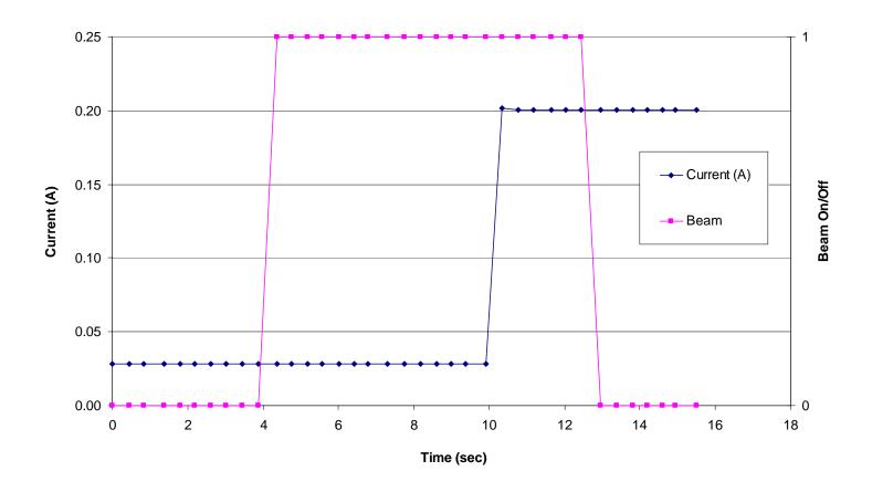
Figure 5.20. Input supply current versus time/fluence for the AD8629 Zero Drift, Single-Supply, Rail-to-Rail, Input/Output Operational Amplifier (run 103, DUT 8, SN12). See Table 4.1 for the details of the test conditions. In this figure the dark blue data points represent the input supply current and the magenta data points represent the beam condition (beam on/beam off). A "0" indicates the shutter is closed (beam off) and a "1" indicates that the shutter is open (beam on).
