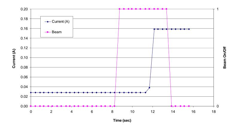
Figure 5.1. Input supply current versus time/fluence for the AD8629 Zero Drift, Single-Supply, Rail-to-Rail, Input/Output Operational Amplifier (run 80, DUT 8, SN12). See Table 4.1 for the details of the test conditions. In this figure the dark blue data points represent the input supply current and the magenta data points represent the beam condition (beam on/beam off). A "0" indicates the shutter is closed (beam off) and a "1" indicates that the shutter is open (beam on).
