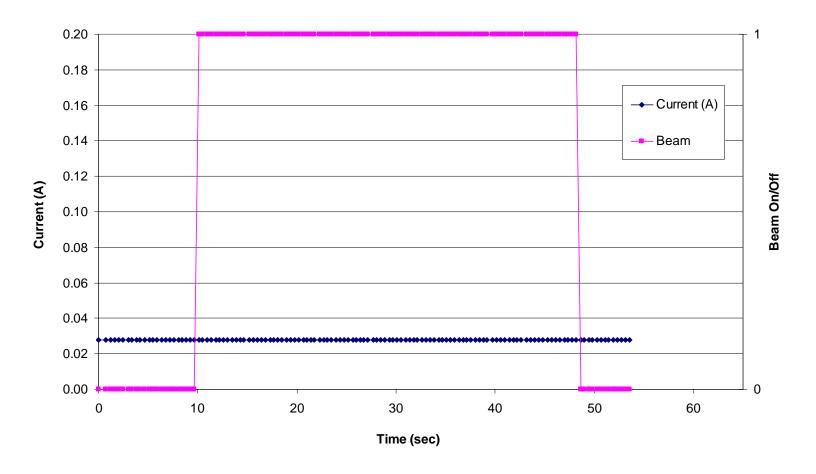
Figure 5.9. Input supply current versus time/fluence for the AD8629 Zero Drift, Single-Supply, Rail-to-Rail, Input/Output Operational Amplifier (run 91, DUT 7, SN11). See Table 4.1 for the details of the test conditions. In this figure the dark blue data points represent the input supply current and the magenta data points represent the beam condition (beam on/beam off). A "0" indicates the shutter is closed (beam off) and a "1" indicates that the shutter is open (beam on).
