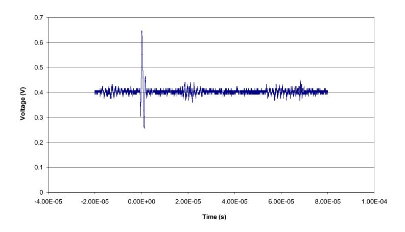
Figure 5.16. Representative single event transient for the AD8629 Zero Drift, Single-Supply, Rail-to-Rail, Input/Output Operational Amplifier (run 102, DUT 8, SN12). The data is presented as output potential versus time/fluence. In this figure the dark blue data points represent the output from the operational amplifier configured in the non-inverting mode. See Table 4.1 for the details of the test conditions.
