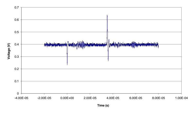
Figure 5.11. Representative single event transient for the AD8629 Zero Drift, Single-Supply, Rail-to-Rail, Input/Output Operational Amplifier (run 93, DUT 5, SN2). The data is presented as output potential versus time/fluence. In this figure the dark blue data points represent the output from the operational amplifier configured in the non-inverting mode. See Table 4.1 for the details of the test conditions.
