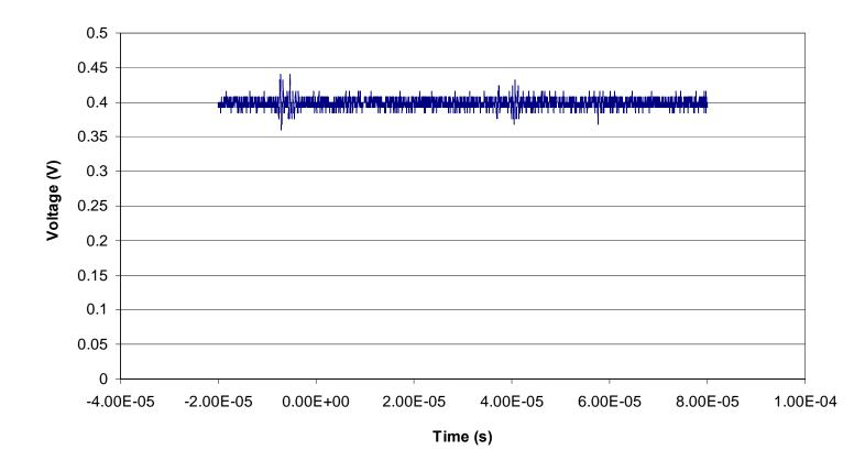
Figure 5.5. Representative single event transient for the AD8629 Zero Drift, Single-Supply, Rail-to-Rail, Input/Output Operational Amplifier (run 86, DUT 5, SN2). The data is presented as output potential versus time/fluence. In this figure the dark blue data points represent the output from the operational amplifier configured in the non-inverting mode. See Table 4.1 for the details of the test conditions.
