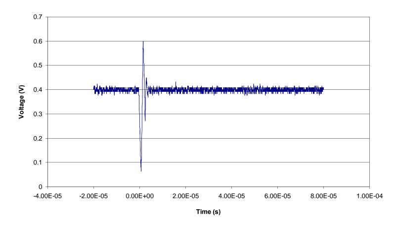
Figure 5.2. Representative single event transient for the AD8629 Zero Drift, Single-Supply, Rail-to-Rail, Input/Output Operational Amplifier (run 83, DUT 6, SN3). The data is presented as output potential versus time/fluence. In this figure the dark blue data points represent the output from the operational amplifier configured in the non-inverting mode. See Table 4.1 for the details of the test conditions.
