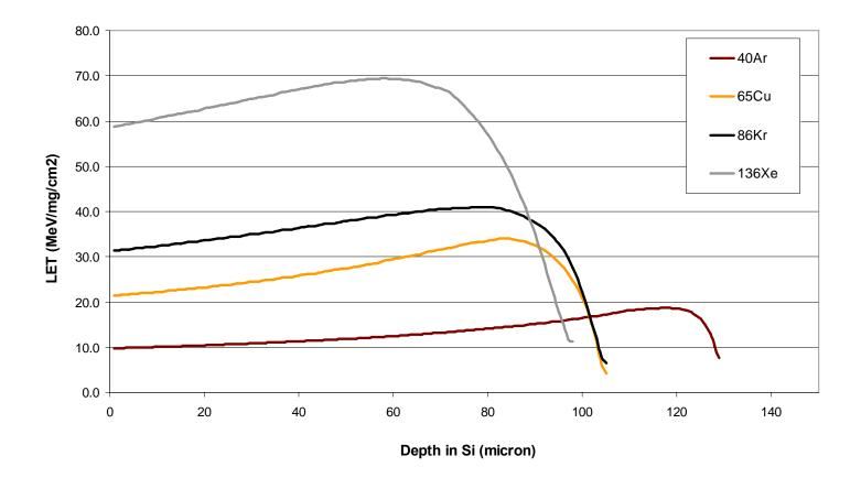
Figure 3.1. Range of the 10MeV/n Xe, Kr, Cu and Ar beams into silicon. The range to the Bragg Peak for Xe (the shortest range ion used) is approximately  $60\mu$ m while the surface LET is approximately 58MeV-cm2/mg.
