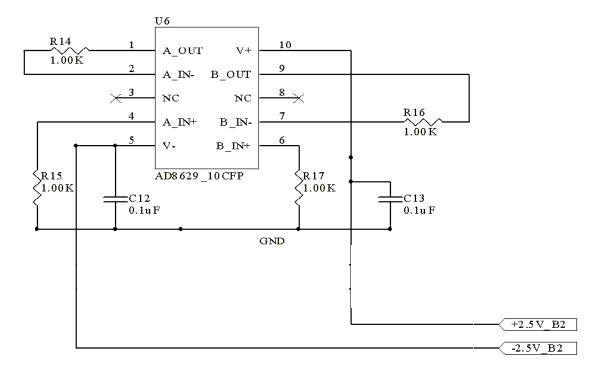
Figure B.1. Schematic drawing of the bias configuration used for the SET test described in this final report.
