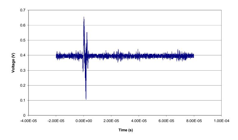
Figure 5.17. Representative single event transient for the AD8629 Zero Drift, Single-Supply, Rail-to-Rail, Input/Output Operational Amplifier (run 107, DUT 7, SN11). The data is presented as output potential versus time/fluence. In this figure the dark blue data points represent the output from the operational amplifier configured in the non-inverting mode. See Table 4.1 for the details of the test conditions.
