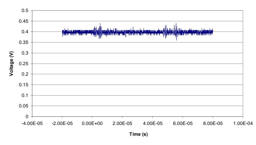
Figure 5.7. Representative single event transient for the AD8629 Zero Drift, Single-Supply, Rail-to-Rail, Input/Output Operational Amplifier (run 89, DUT 7, SN11). The data is presented as output potential versus time/fluence. In this figure the dark blue data points represent the output from the operational amplifier configured in the non-inverting mode. See Table 4.1 for the details of the test conditions.
