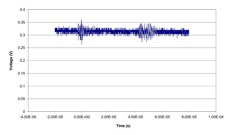
Figure 5.13. Representative single event transient for the AD8629 Zero Drift, Single-Supply, Rail-to-Rail, Input/Output Operational Amplifier (run 95, DUT 5, SN2). The data is presented as output potential versus time/fluence. In this figure the dark blue data points represent the output from the operational amplifier configured in the non-inverting mode. See Table 4.1 for the details of the test conditions.
