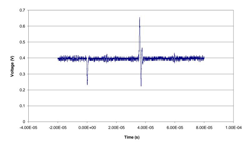
Figure 5.8. Representative single event transient for the AD8629 Zero Drift, Single-Supply, Rail-to-Rail, Input/Output Operational Amplifier (run 90, DUT 7, SN11). The data is presented as output potential versus time/fluence. In this figure the dark blue data points represent the output from the operational amplifier configured in the non-inverting mode. See Table 4.1 for the details of the test conditions.
