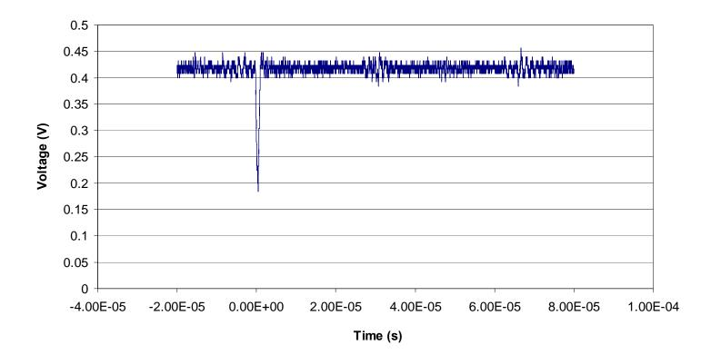
Figure 5.4. Representative single event transient for the AD8629 Zero Drift, Single-Supply, Rail-to-Rail, Input/Output Operational Amplifier (run 85, DUT 5, SN2). The data is presented as output potential versus time/fluence. In this figure the dark blue data points represent the output from the operational amplifier configured in the non-inverting mode. See Table 4.1 for the details of the test conditions.
