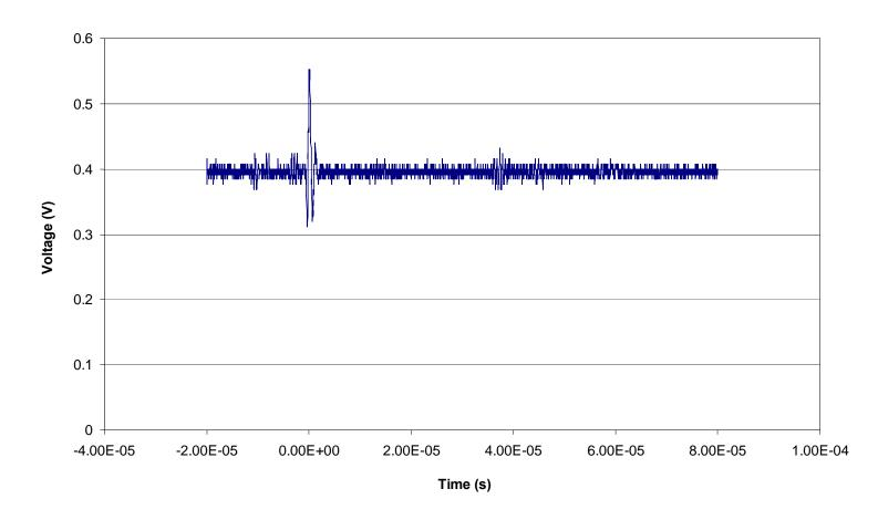
Figure 5.9. Representative single event transient for the AD8629 Zero Drift, Single-Supply, Rail-to-Rail, Input/Output Operational Amplifier (run 91, DUT 7, SN11). The data is presented as output potential versus time/fluence. In this figure the dark blue data points represent the output from the operational amplifier configured in the non-inverting mode. See Table 4.1 for the details of the test conditions.
