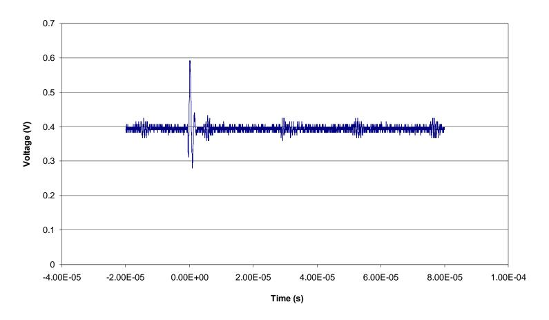
Figure 5.12. Representative single event transient for the AD8629 Zero Drift, Single-Supply, Rail-to-Rail, Input/Output Operational Amplifier (run 94, DUT 5, SN2). The data is presented as output potential versus time/fluence. In this figure the dark blue data points represent the output from the operational amplifier configured in the non-inverting mode. See Table 4.1 for the details of the test conditions.
