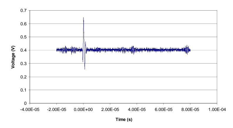
Figure 5.14. Representative single event transient for the AD8629 Zero Drift, Single-Supply, Rail-to-Rail, Input/Output Operational Amplifier (run 100, DUT 8, SN12). The data is presented as output potential versus time/fluence. In this figure the dark blue data points represent the output from the operational amplifier configured in the non-inverting mode. See Table 4.1 for the details of the test conditions.
