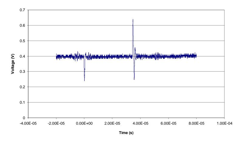
Figure 5.6. Representative single event transient for the AD8629 Zero Drift, Single-Supply, Rail-to-Rail, Input/Output Operational Amplifier (run 88, DUT 5, SN2). The data is presented as output potential versus time/fluence. In this figure the dark blue data points represent the output from the operational amplifier configured in the non-inverting mode. See Table 4.1 for the details of the test conditions.
