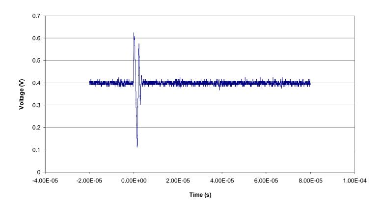
Figure 5.3. Representative single event transient for the AD8629 Zero Drift, Single-Supply, Rail-to-Rail, Input/Output Operational Amplifier (run 84, DUT 5, SN2). The data is presented as output potential versus time/fluence. In this figure the dark blue data points represent the output from the operational amplifier configured in the non-inverting mode. See Table 4.1 for the details of the test conditions.
