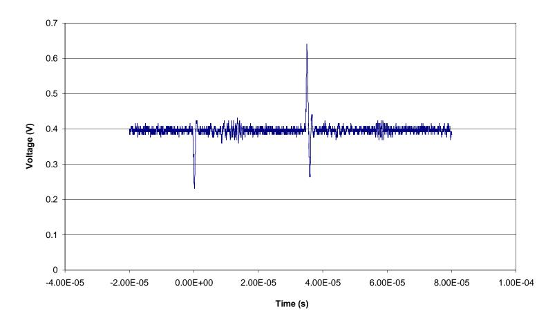
Figure 5.10. Representative single event transient for the AD8629 Zero Drift, Single-Supply, Rail-to-Rail, Input/Output Operational Amplifier (run 92, DUT 5, SN2). The data is presented as output potential versus time/fluence. In this figure the dark blue data points represent the output from the operational amplifier configured in the non-inverting mode. See Table 4.1 for the details of the test conditions.
