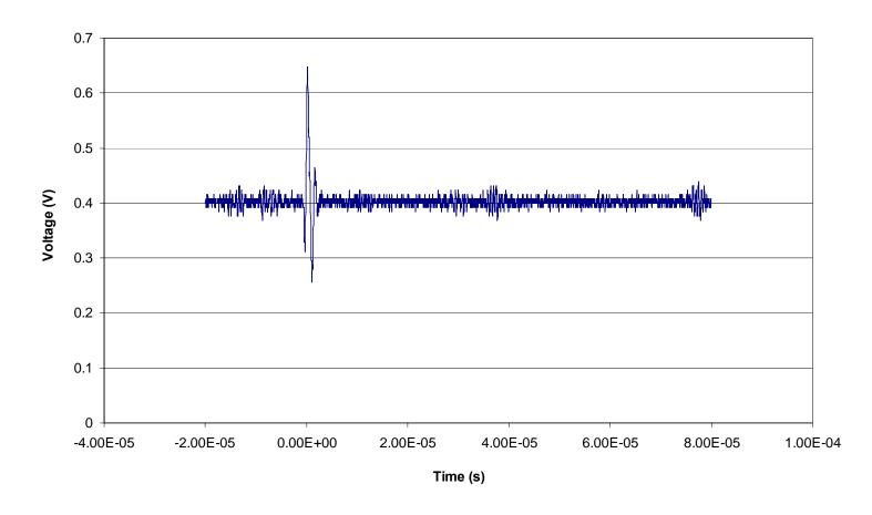
Figure 5.15. Representative single event transient for the AD8629 Zero Drift, Single-Supply, Rail-to-Rail, Input/Output Operational Amplifier (run 101, DUT 8, SN12). The data is presented as output potential versus time/fluence. In this figure the dark blue data points represent the output from the operational amplifier configured in the non-inverting mode. See Table 4.1 for the details of the test conditions.
