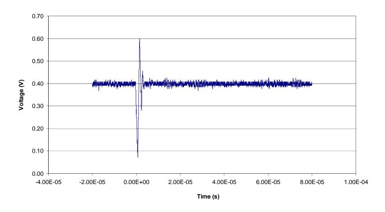
Figure 5.1. Representative single event transient for the AD8629 Zero Drift, Single-Supply, Rail-to-Rail, Input/Output Operational Amplifier (run 80, DUT 8, SN12). The data is presented as output potential versus time/fluence. In this figure the dark blue data points represent the output from the operational amplifier configured in the non-inverting mode. See Table 4.1 for the details of the test conditions.
