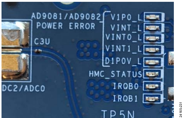
Figure 32. LEDs Denoting Power to the Various Rails on the Evaluation Board
