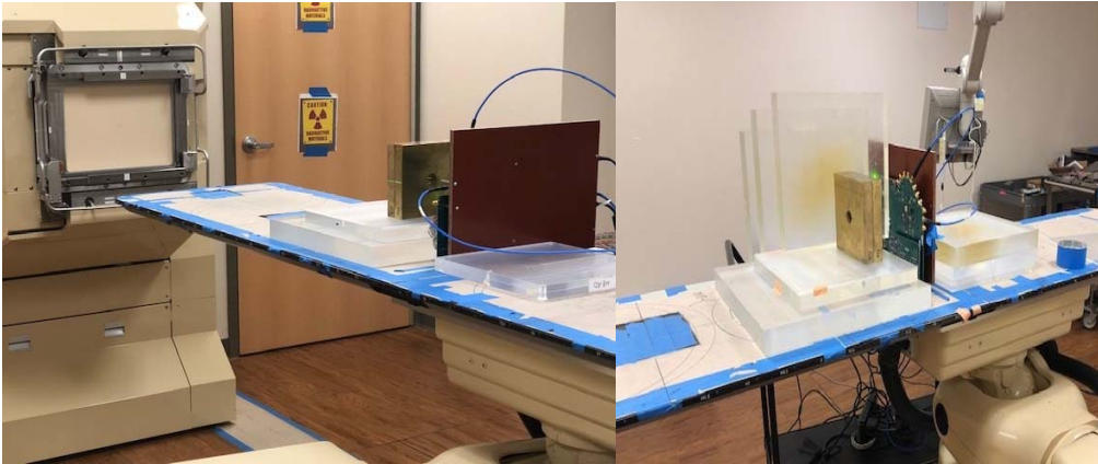
Figure 3 AD9213 proton test setup
