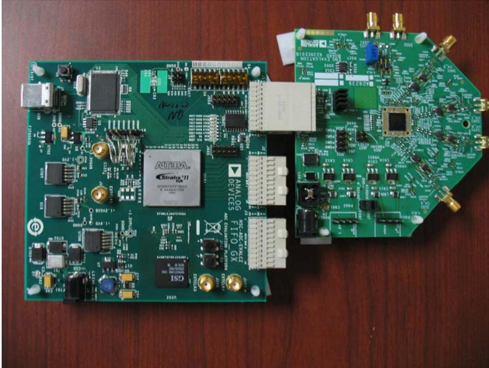
**Figure 1: AD9239 Evaluation Board – HSC\_ADC\_EVALC FIFO\_GX Data Capture Board**
