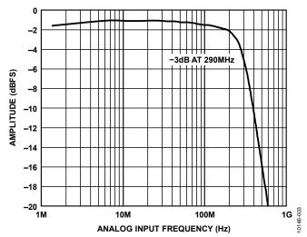
Figure 3. Pass-Band Flatness Performance vs. Frequency
