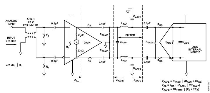
Figure 5. Generalized Differential Amplifier/ADC Interface with Low-Pass Filter
