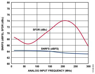
Figure 4. SNR/SFDR Performance vs. Frequency
