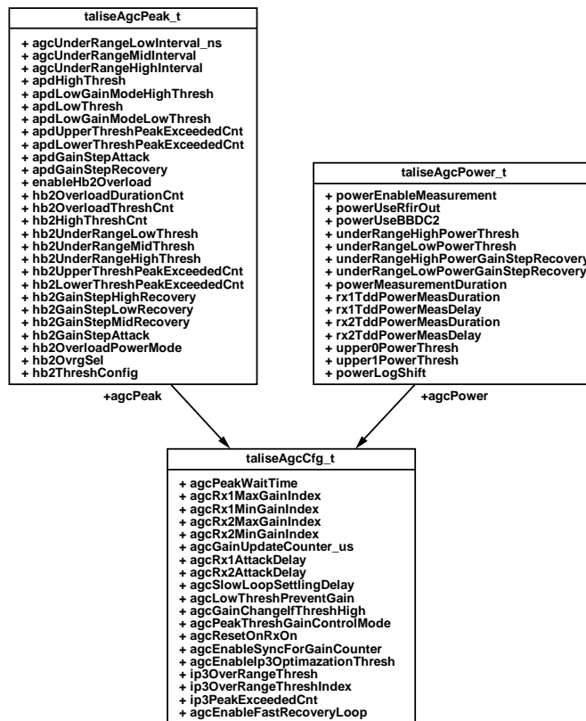
Figure 90. Member Listing of taliseAgcCfg_t, taliseAgcPeak_t, and taliseAgcPower_t Data Structures
