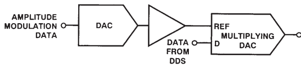
Figure 6. Amplitude Modulation Using a Multiplying DAC
