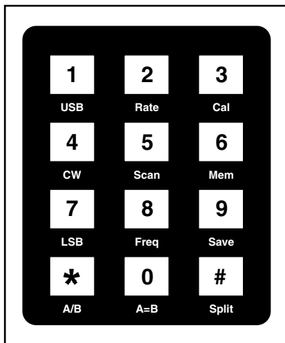
Figure 9. Keypad Overlay for Reproduction, 47 mm Wide by 57.5 mm High
