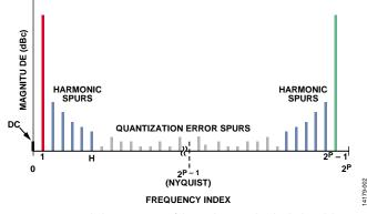
Figure 2. Spectral Characteristics of the Angle to Amplitude Block and the DAC
