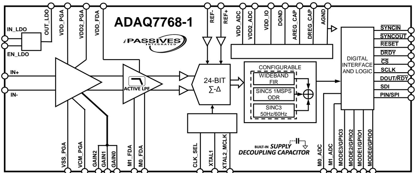
Figure 1. Block Diagram
