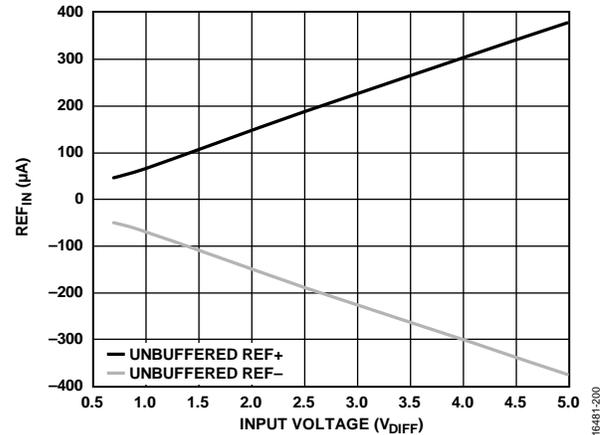
Figure 73. Reference Input Current (REF<sub>IN</sub>) vs. Input Voltage, Unbuffered REF+ and REF-
