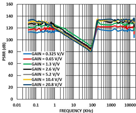
Figure 52. VDD\_PGA AC PSSR across All Gains, using the Internal Supply Decoupling Capacitor
