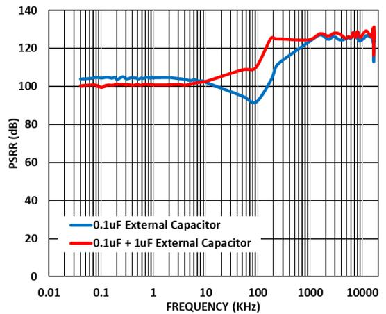
Figure 54. VDD\_IO using External Supply Decoupling Capacitor
