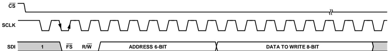
Figure 99. 3-Wire SPI Write Frame ( $\overline{\text{CS}} = 0$ )
