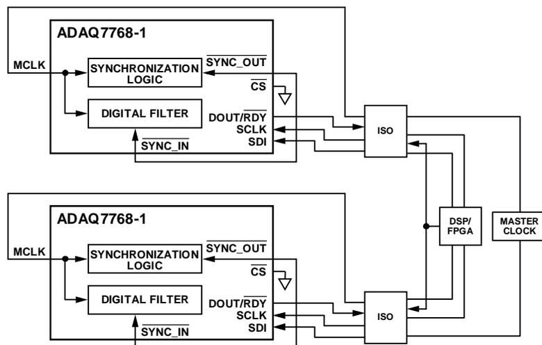
Figure 107. Synchronization in Channel to Channel Isolated Systems
