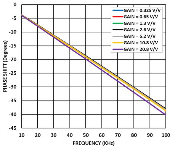
Figure 40. Analog Front End (AFE) Phase Response
