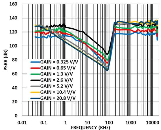
Figure 53. VSS\_PGA AC PSSR across All Gains, using the Internal Supply Decoupling Capacitor
