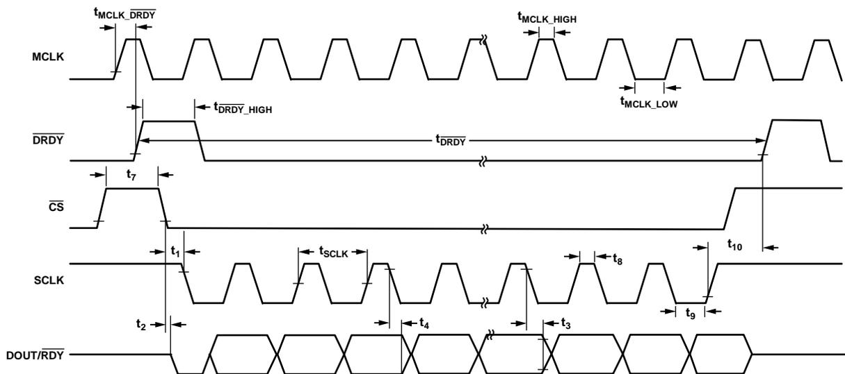
Figure 102. Serial Interface Timing Diagram, Example Reflects Reading an ADC Conversion in Continuous Read Mode
