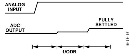
Figure 89. Sinc3 Filter Step Response
