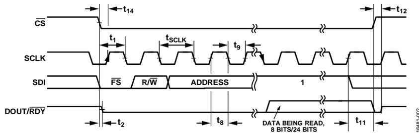
Figure 2. SPI Read Timing Diagram
