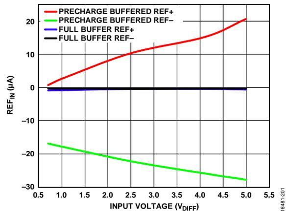
Figure 74. Reference Input Current (REF<sub>IN</sub>) vs. Input Voltage, Precharge Buffered REF+ and REF- and Full Buffer REF+ and REF-
