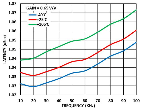
Figure 42. Analog Front End (AFE) Latency vs Frequency across Temperature, Gain = 0.65 V/V
