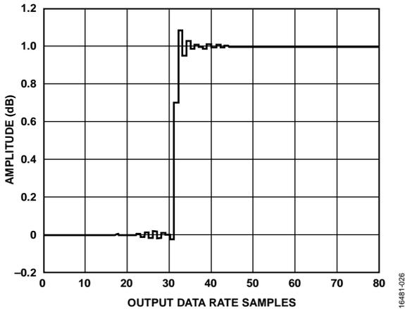
Figure 84. Wideband Low Ripple FIR Filter Step Response
