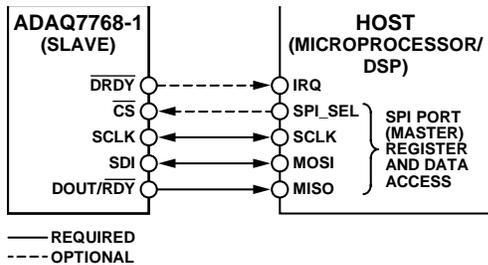
Figure 96. Basic Serial Port Connection Diagram
