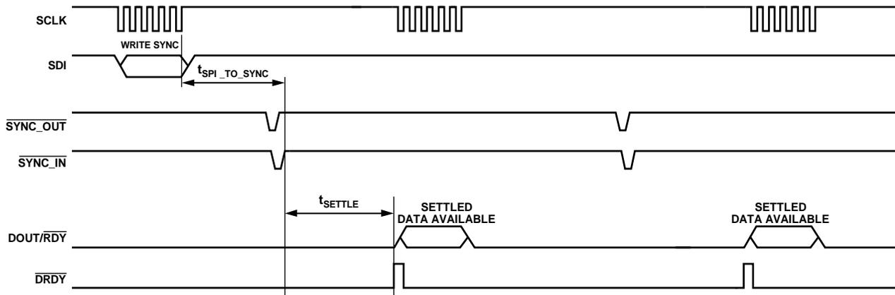
Figure 106. One Shot Conversion Mode,  $\overline{\text{SYNC\_IN}}$  Pulse Initiated by a Register Write
