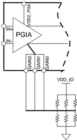
Figure 10. PGIA Gain Control using External Resistors
