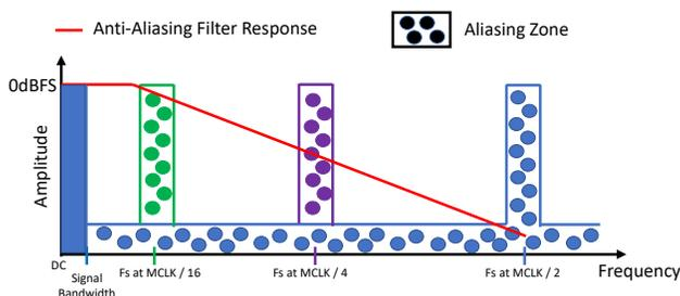
Figure 91. Anti-Alias Filter Response versus MCLK Divider
