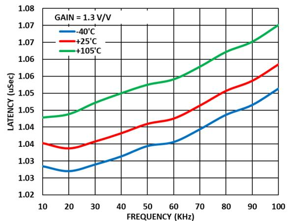
Figure 43. Analog Front End (AFE) Latency vs Frequency across Temperature, Gain = 1.3 V/V
