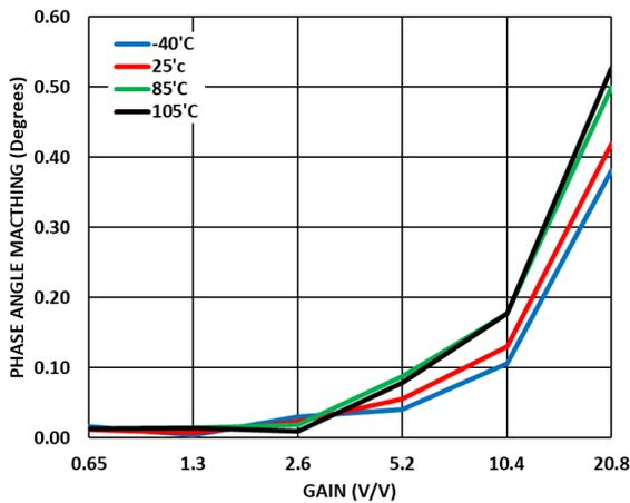
Figure 39. Phase Matching vs PGA Gain over Temperature, Normalized to Gain = 0.325 V/V
