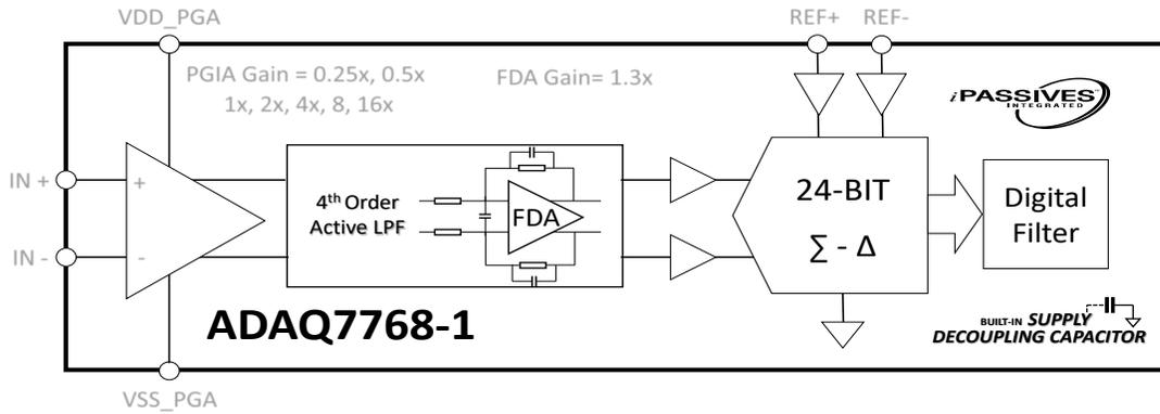
Figure 65. ADAQ7768-1 Top Level Core Signal Chain
