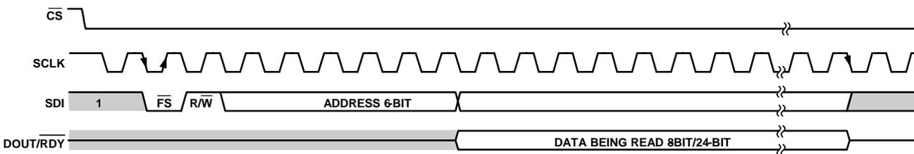
Figure 100. 3-Wire SPI Read Frame ( $\overline{\text{CS}} = 0$ )
