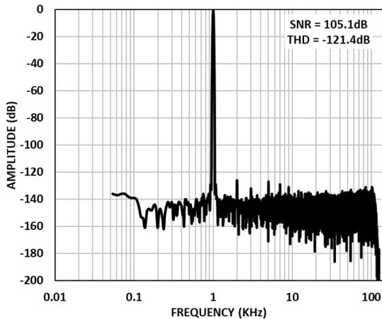
Figure 15. FFT Wideband Low Ripple FIR Filter, Differential Input, -0.5dBFS, Gain = 0.65 V/V, FDA = Full Power.
