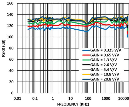
Figure 51. LDO AC PSSR across All Gains, connected to VDD2\_PGA, VDD\_FDA, VDD\_ADC, VDD2\_ADC with Internal Supply Decoupling Capacitor
