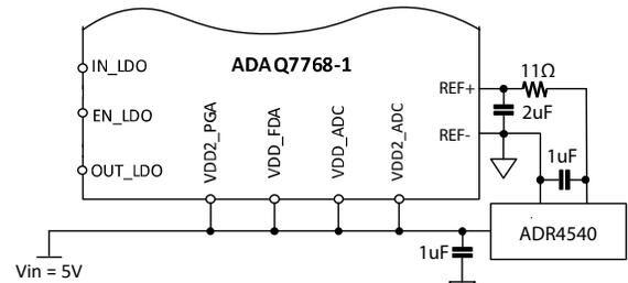
Figure 77. Float IN\_LDO and OUT\_LDO pins when not used
