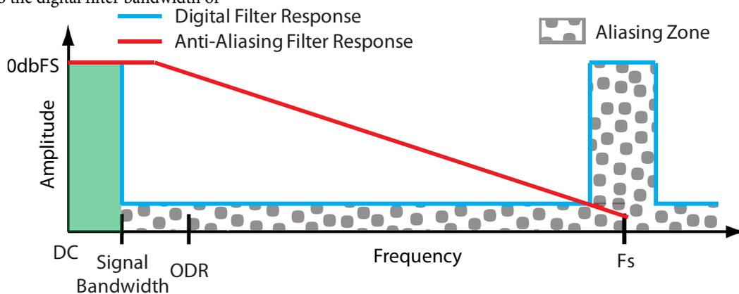
Figure 66. Simplified illustration of the overall frequency response
