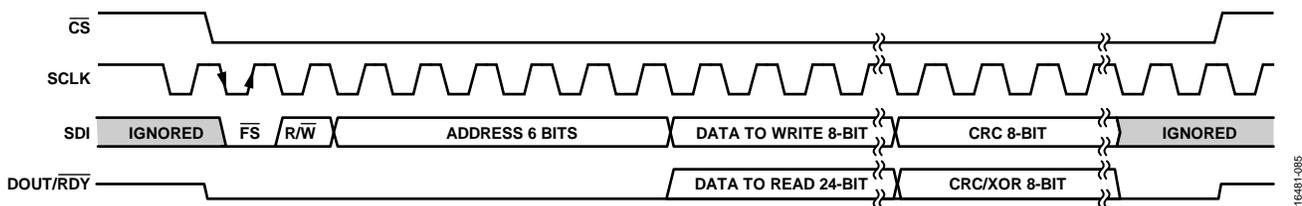
Figure 101. Data Output Format When Using CRC
