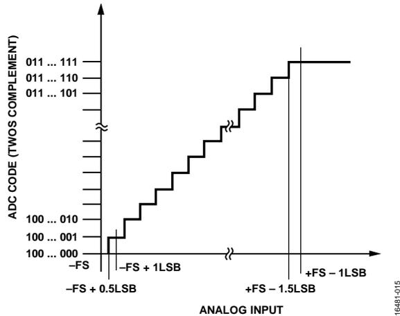
Figure 75. ADC Ideal Transfer Functions (FS is Full-Scale)
