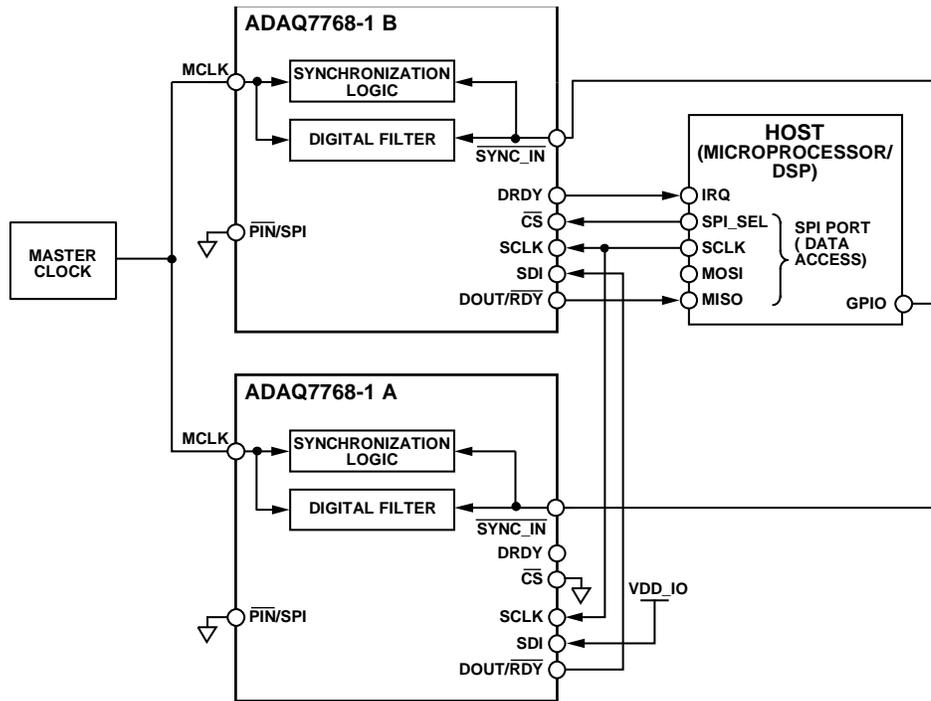
Figure 93. Daisy-Chaining Multiple ADAQ7768-1 Devices
