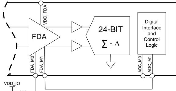
Figure 72. FDA Full Power Mode Connection
