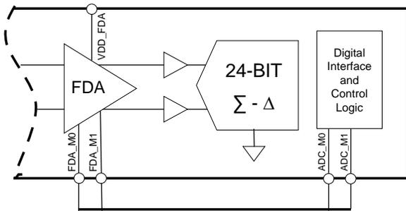
Figure 71. FDA Eco Power Mode Connection
