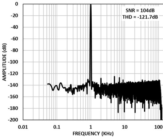
Figure 20. FFT Wideband Low Ripple FIR Filter, Bipolar Single Ended Input, -0.5dBFS, Gain = 1.3 V/V, FDA = Full Power.
