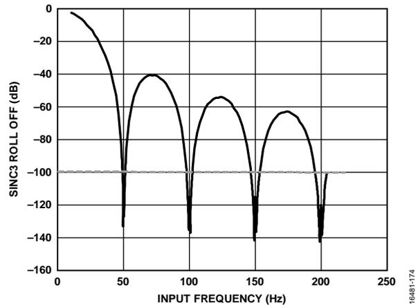
Figure 90. Sinc3 Filter Frequency Response Showing 50 Hz Rejection, 50 Hz ODR, ×163,840 Decimation
