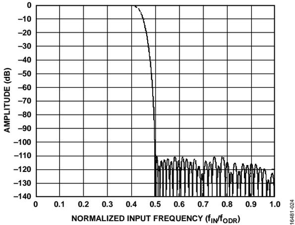
Figure 82. Low Ripple FIR Filter Frequency Response
