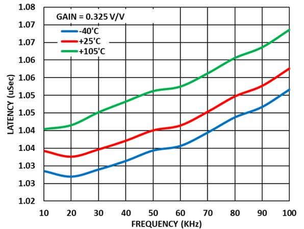
Figure 41. Analog Front End (AFE) Latency vs Frequency across Temperature, Gain = 0.325 V/V
