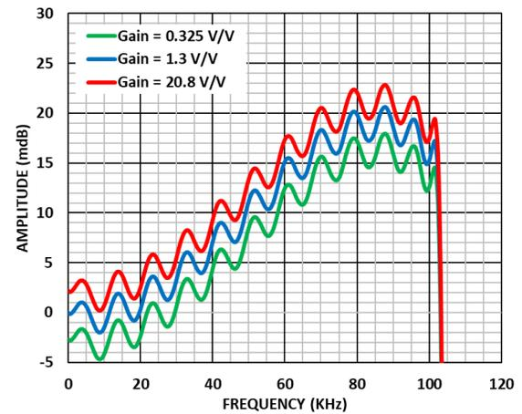
Figure 49. ADAQ7768-1 Wideband Low Ripple FIR Filter Pass-Band Ripple, ODR = 256 kSPS, Normalized to Gain = 1.3 V/V
