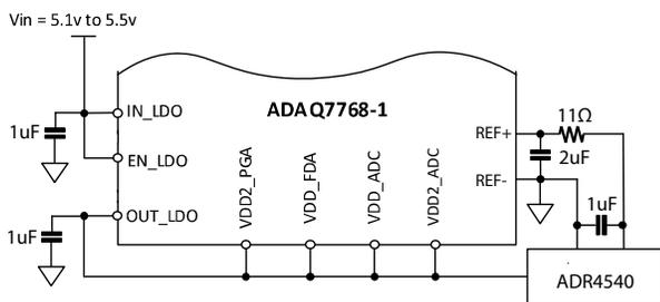
Figure 76. ADAQ7768-1 power supply connection using internal LDO
