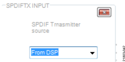
Figure 43. Routing the DSP Core Outputs to the S/PDIF Transmitter
