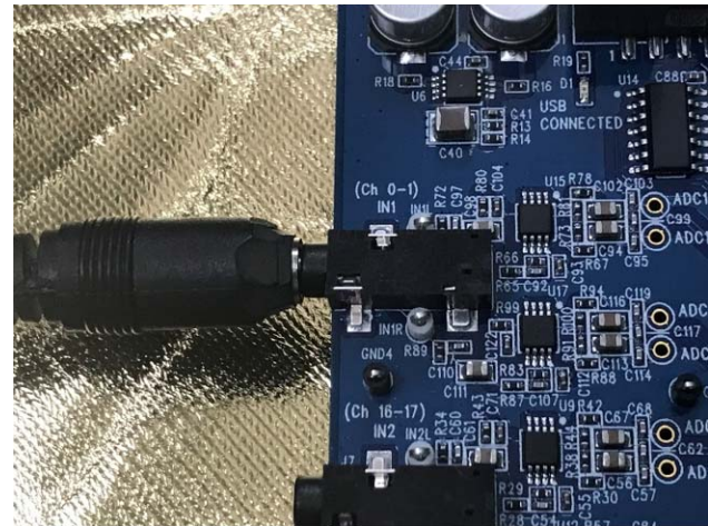
Figure 11. Analog Stereo Input Source Connection at J9 (IN1)
