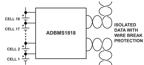
Figure 1. Typical Application Circuit
