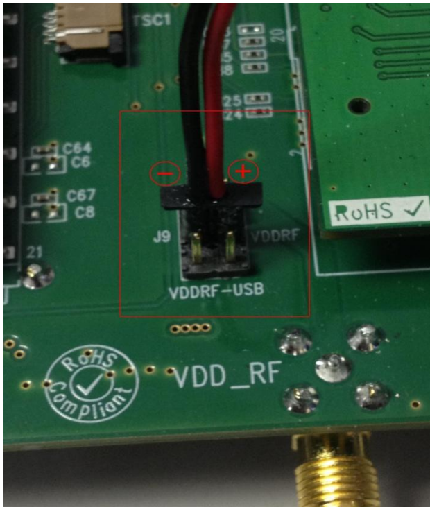
Figure 44 (Powering the ADF7023 Directly from Header J9)
