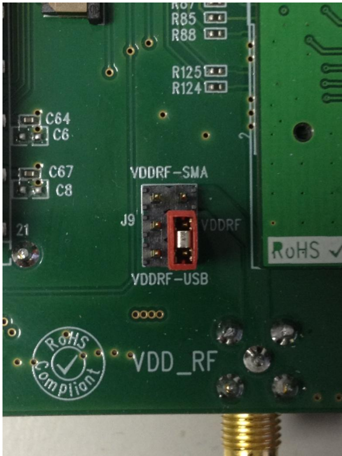
Figure 42 (Default Jumper configuration)
