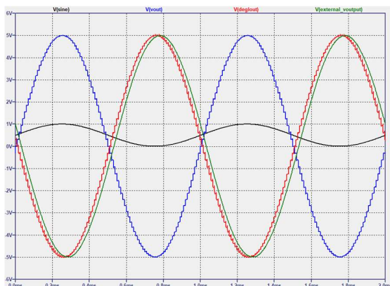
Figure 8.- TRAN example: 1 kHz input sinewave, 100 kps
