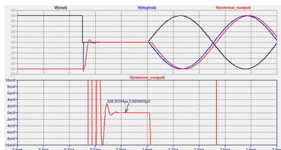
Figure 6.-TRAN example: 5V step and sinewave settling
