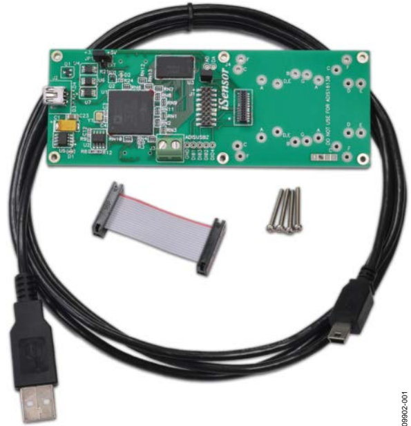
Figure 1. Photograph of Inertial Sensor Evaluation System
