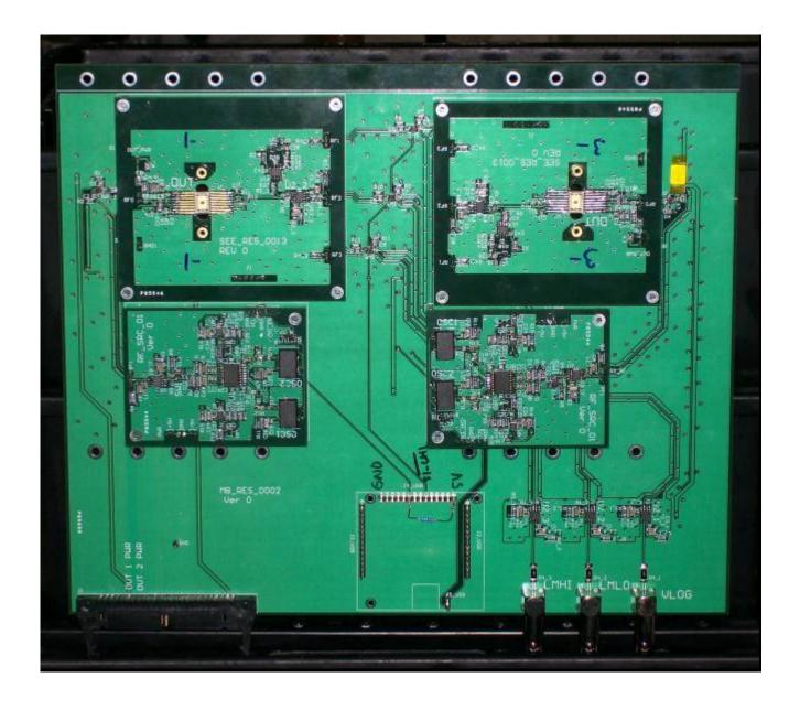
Figure 3.1. Single event test board prepared for mounting on the test stage at TAMU. The board has two units-under-test mounted simultaneously to minimize interruptions during testing. There is also a heater plate mounted to the backside of the daughter cards to provide the elevated temperature required for this testing. Also seen on the motherboard are two custom RF source daughter cards used to supply clean 5MHz or 10MHz signals to the units-under-test.
