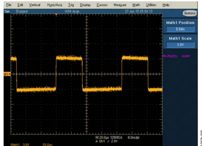
Figure 9. Math Y – Z Waveform for the RS-485 Port on the EVAL-CN0373-EB1Z Board
