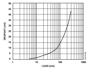
Figure 6. Dropout Voltage vs. Load Currents ( $I_{LOAD}$ )  $V_{OUT} = 2.5 \text{ V}, T_A = 25 ^{\circ}\text{C}$
