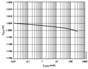
Figure 5. Output Voltage,  $V_{OUT}$  vs. Load Current,  $I_{OUT}$  at  $V_{IN}$  = 2.3 V,  $V_{OUT}$  = 1.8 V,  $T_A$  = 25°C
