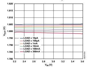
Figure 4. Output Voltage ( $V_{OUT}$ ) vs. Input Voltage ( $V_{IN}$ ) at  $T_A = 25$ °C
