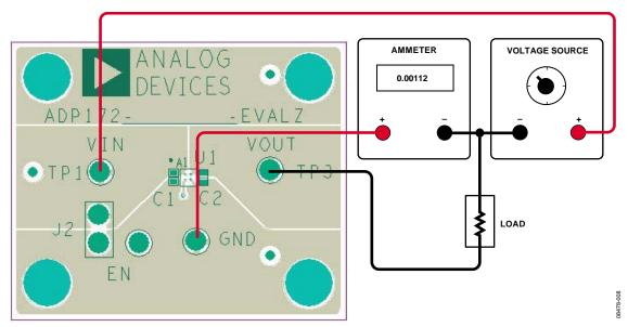
Figure 8. Ground Current Measurement Setup, WLCSP
