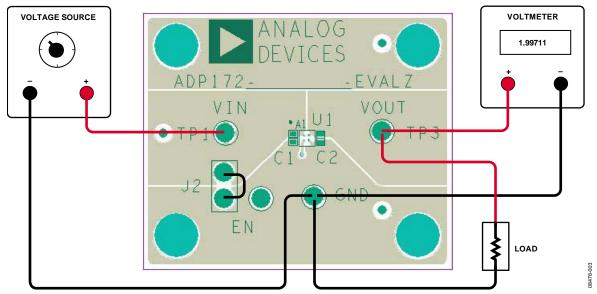
Figure 3. Output Voltage Measurement Setup, WLCSP
