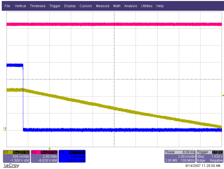
Figure 17. Output Disable; Ch1 = 1.2V @ 0A, Ch2 = V_{IN} @ 12.6 V, Ch3 = Enable
