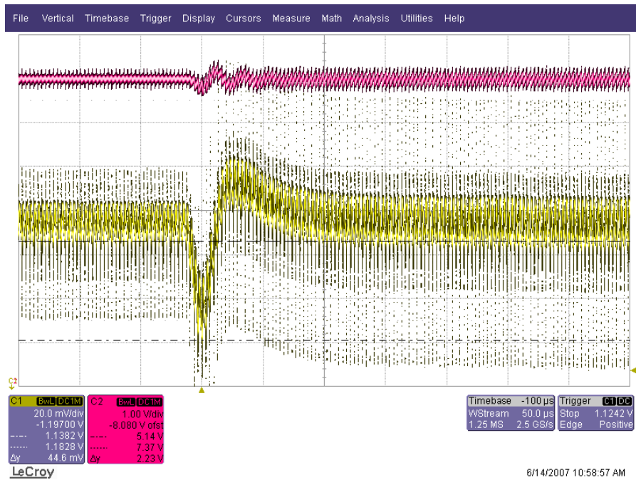
Figure 8. Load Transient; Ch1 = 1.2V @ 5-15 A 1 A/us, Ch2 = V_{IN} @ 11.04 V
