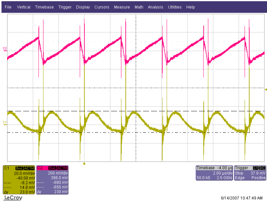
Figure 5. Voltage Ripple; Ch1 = 1.2 V @ 20 A, Ch2 = V_{IN} @ 12.6 V
