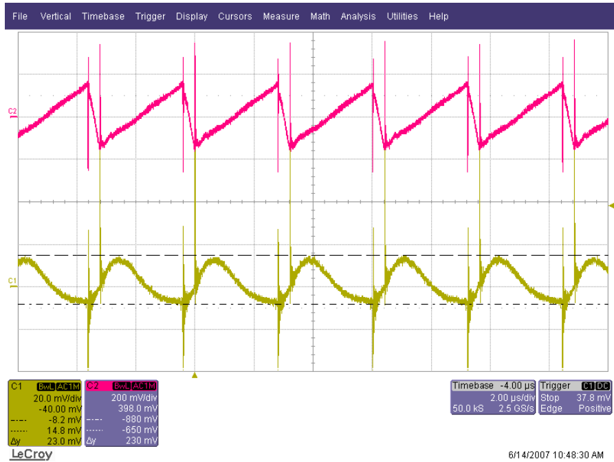
Figure 7. Voltage Ripple; Ch1 = 1.2V @ 20 A, Ch2 = V_{IN} @ 11.04 V
