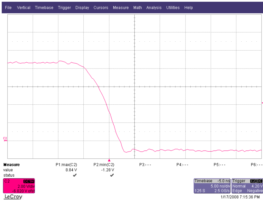
Figure 18. Switchnode Falling 100% load Vin @ 9 V: Ch2 = Drain to Source of QL1
