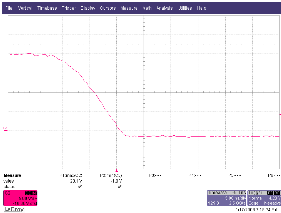
Figure 20. Switchnode Falling 100% load Vin @ 20 V: Ch2 = Drain to Source of QL1
