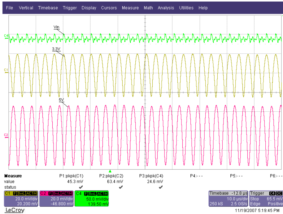
Figure 13. Switching regulator ripple and noise at no load: Ch1 = 3.3 V, Ch2 = 5.0 V, Ch4 = Vin @ 16.0 V
