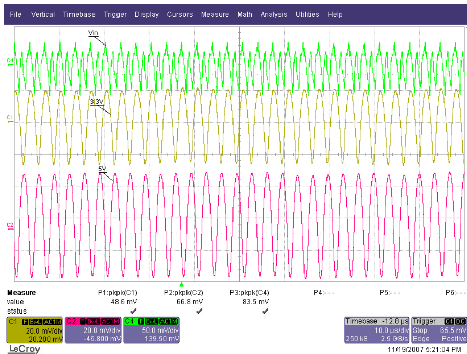
Figure 14. Switching regulator ripple and noise at full load: Ch1 = 3.3 V, Ch2 = 5.0 V, Ch4 = Vin @ 16.0 V
