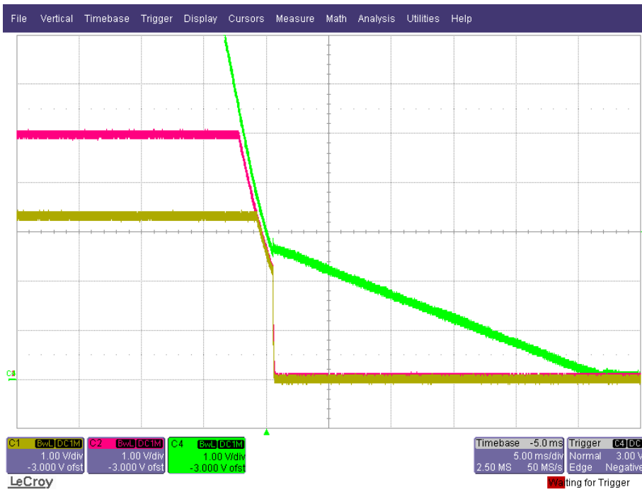
Figure 10. Switching regulator turn off at full load: Ch1 = 3.3 V, Ch2 = 5.0 V, Ch4 = Vin
