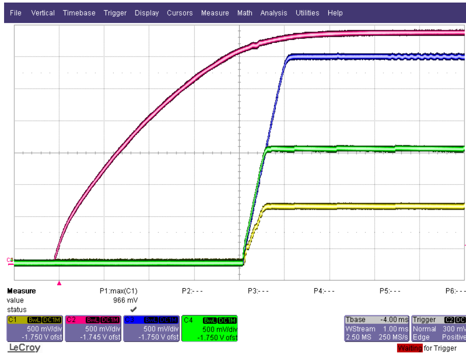
Figure 6. Switching regulator turn on at no load: Ch1 = 0V9_FPGA, Ch2 = Vo3V6, Ch3 = 3V3_DCD, Ch4 = 1V8_DCD
