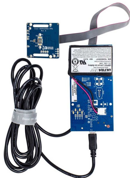
Figure 5. Connect the EVAL-ADPDUCZ to the EVAL-ADPD4200Z-PPG
