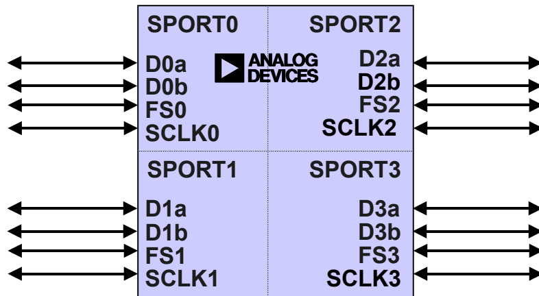
Figure 16. ADSP-21161 SPORTs Pins
