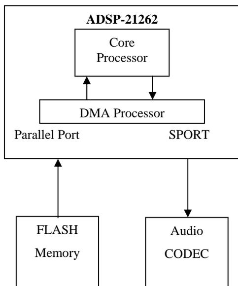
*Figure 2. Data I/O Scheme for the SHARC-based MP3 Decoder*
