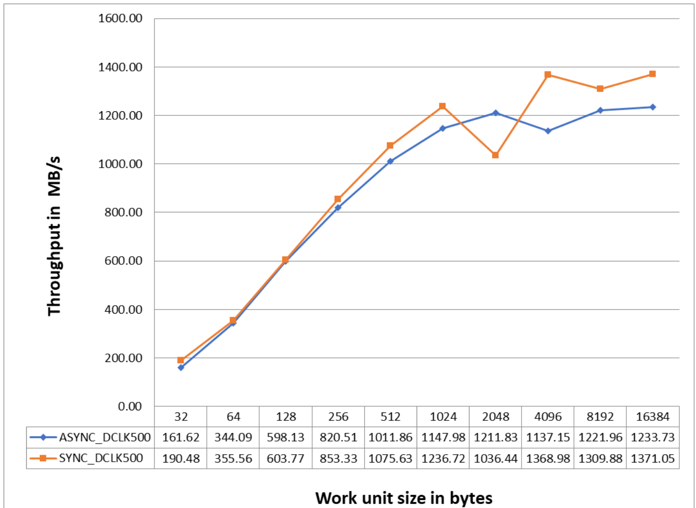
Figure 9: DMC MDMA Throughput with and Without IBx Sync Mode Programming
