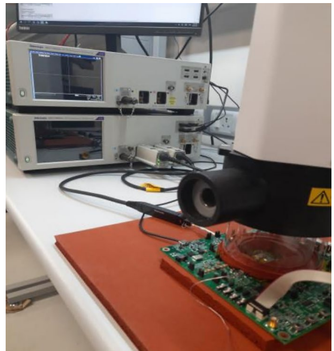
Figure 6. DDR3L Compliance Testing Setup
