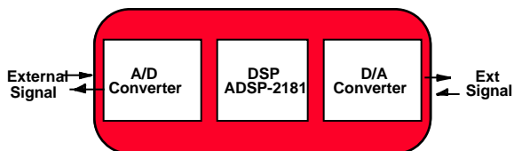
Figure 1 - DSP Data Flow
