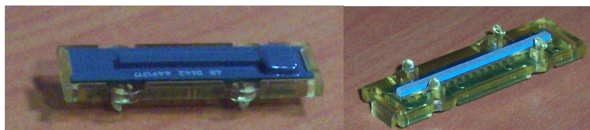
Figure 3. AT77C104B sensor IC with holder and elastomer connector
