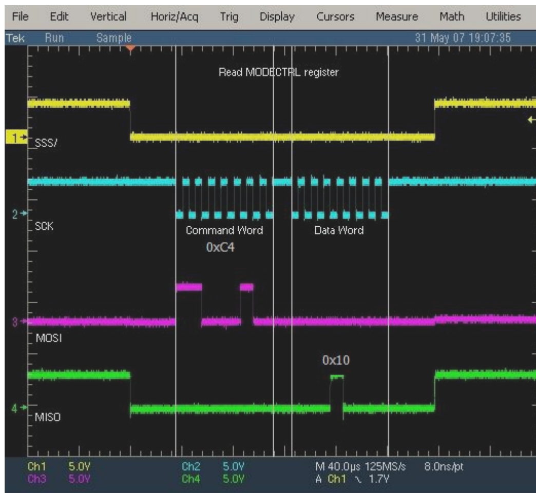
Figure 15. Read MODECTRL register
