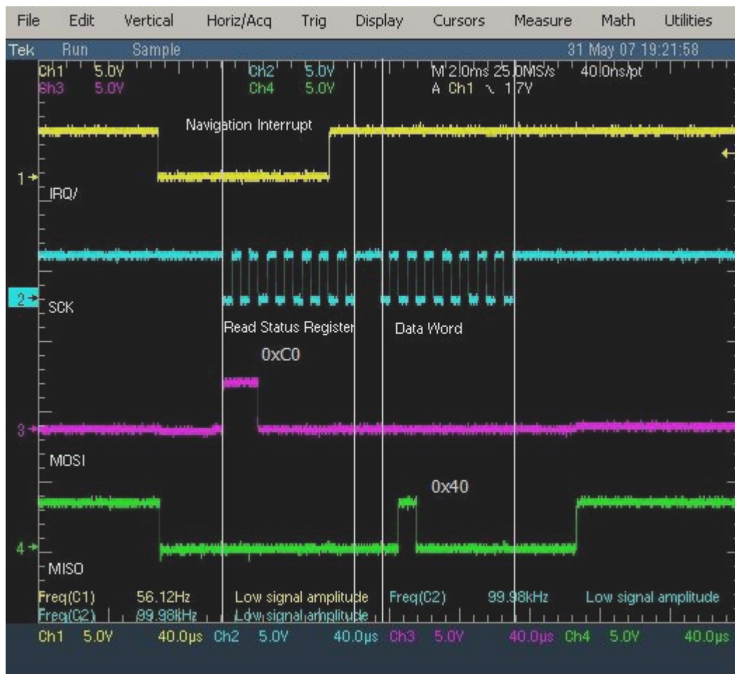
Figure 17. Navigation interrupt and read status register
