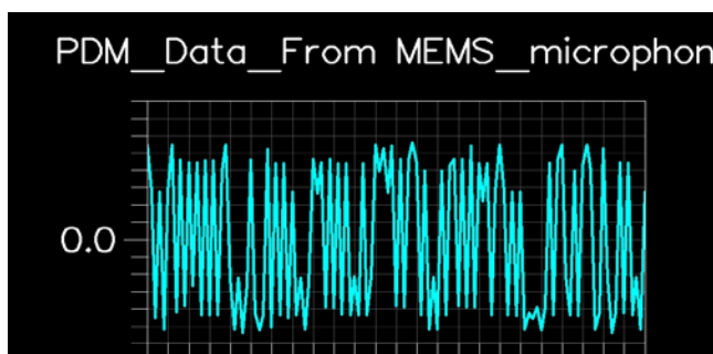
Figure 8. PDM data coming out of microphone
