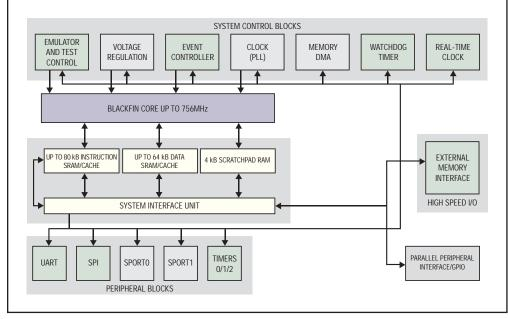
Blackfin Processors integrate an array of peripherals designed to simplify board development and minimize overall system costs.
