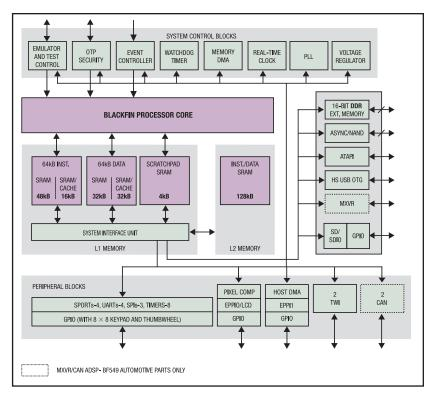
automotive) interfaces provide glueless interfaces to multiple off-chip devices, including consumer and communication products, Bluetooth, and other application-specific interfaces. This level of integration is perfect for the emerging and constantly changing products and standards in the car infotainment and multimedia segments.
