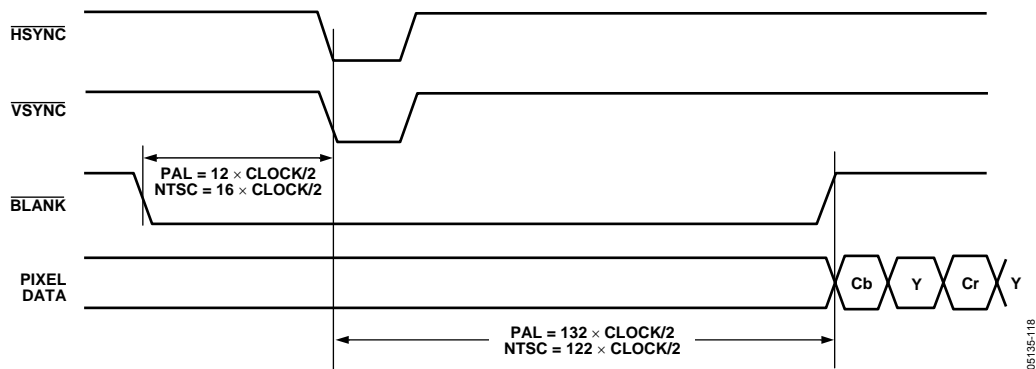
Figure 117. SD Timing Mode 2 Even-to-Odd Field Transition Master/Slave
