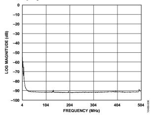
Figure 6. CVBS Measured at the Output of the ADA4432-1, PLL Off, 2× Oversampling, Low Output Drive Mode
