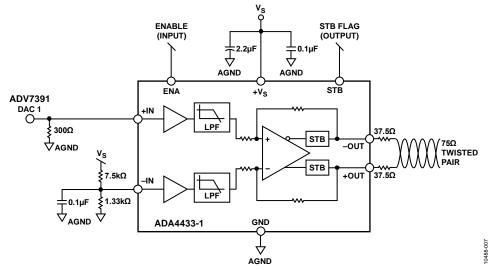
Figure 7. ADA4433-1 Typical Application Circuit
