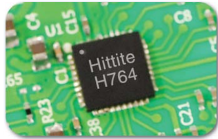
HMC764LP6CE PLL with Integrated VCO on Hittite's Evaluation PCB
