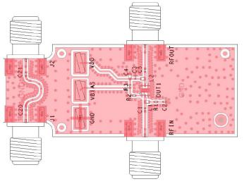
Figure 5. EV1HMC8413LP2F Assembly Drawing (J1 and J2 are Not Installed)
