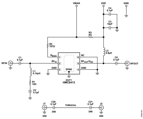
Figure 4. EV1HMC8413LP2F Schematic
