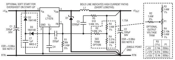
NOTE 1: DO NOT SUBSITTUTE COMPONENTS WITHOUT COMPLETE EVALUATION. NOTE 2: C1 AND C2 MUST BE  $0.07\Omega$  MIN ESR AT ROOM TEMPERATURE (25°C). UNITED CHEMICON SXE50VB331M10X30LL, SPRAGUE 672D337F020DM4D.
